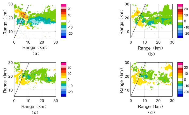
**Figure 5.** Plan Position Indicator (PPI) scans of radial wind speed (m/s) at (a) 0.5°; (b) 2.9°; (c) 5.3°; (d) 6.5° elevations at 20:23–20:25 UT on 30 July 2017. Black lines represent the radar radial line.
