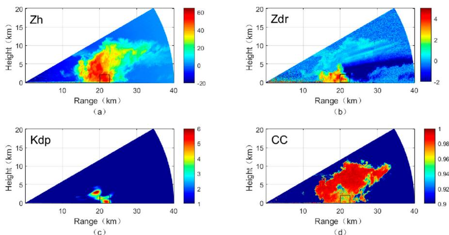
**Figure 6.** Range–Height Indicator (RHI) scans of dual-polarization variables: (a)  $Z_h$ ; (b)  $Z_{dr}$ ; (c)  $K_{dp}$ ; and (d) correlation coefficient (CC) at azimuth of 31° at 20:28 UT on 30 July 2017. Black box indicates the critical area in which the downburst was generated.
