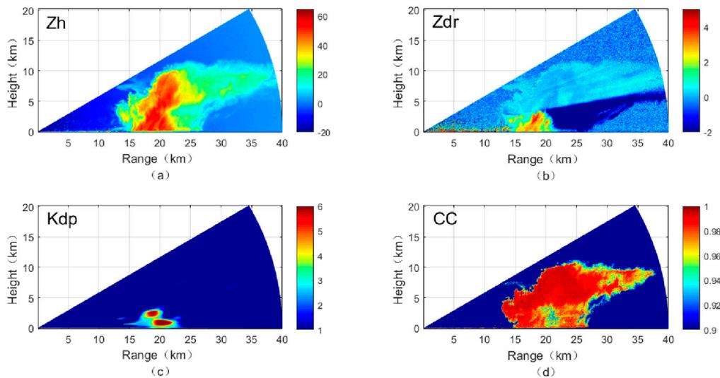
**Figure 7.** RHI scans of dual-polarization variables of (a)  $Z_h$ ; (b)  $Z_{dr}$ ; (c)  $K_{dp}$ ; and (d) CC at the azimuth of  $37^\circ$  at 20:32 UT on 30 July 2017.
