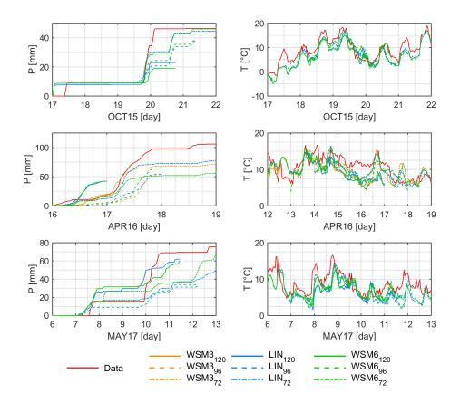
**Figure 5.** Observed and simulated precipitation (**left**) and temperature (**right**) time series for OCT15 (**upper** row), APR16 (**central** row) and MAY17 (**lower** row) events. Three lead times (72, 96 and 120 h) and three MP parameterizations (LIN, WSM6 and WSM3 when used) are considered. Graphical modifications to the rainfall time series are indicated in the previous paragraphs.
