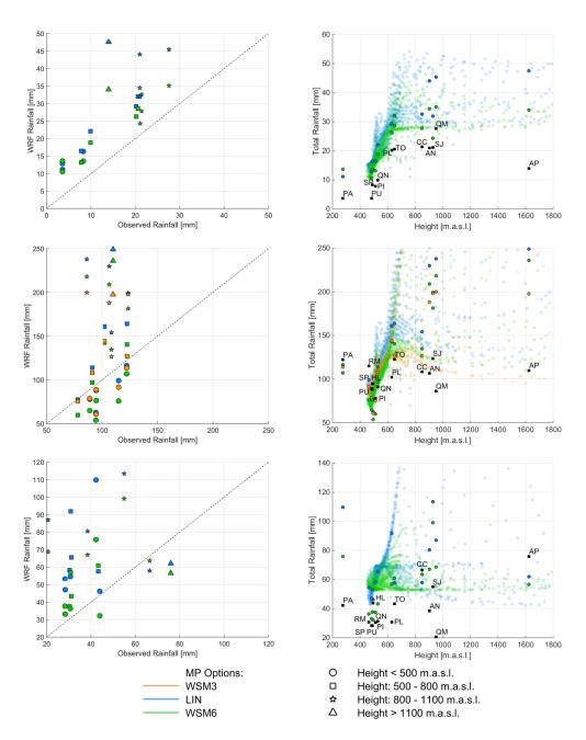
**Figure 4.** Total observed and simulated precipitation according to height (**left**) and orographical gradient (**right**) for OCT15 (**upper** row), APR16 (**central** row) and MAY17 (**lower** row) events. The mean value of all lead times (72, 96 and 120 h) and three MP parameterizations (LIN, WSM6 and WSM3 when used) are considered. In right panels, observed data are plotted in black squares.
