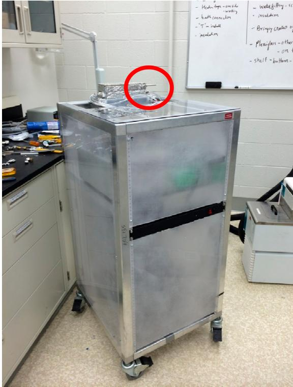
**Figure S9:** Photograph of the chamber 2 as described in Figure 1. Highlighted unit of the chamber shows the inlet port.
