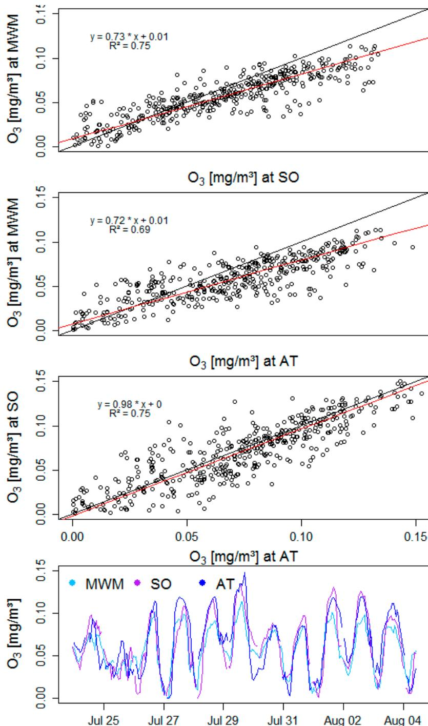
**Figure S1.** Scatter plots (1-3 from top) with correlation line (red), 1:1 line (black), linear fit, and coefficient of determination for the respective ozone concentrations. Top panel Allertal (AT) and Mittleres Wietingsmoor (MWM), second panel from top Südoldenburg (SO) and MWM, third panel AT and SO. The bottom panels shows time series of ozone concentrations at the three sites.
