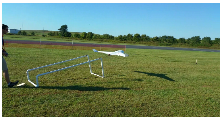
Figure 1. BLUECAT5 takeoff with launcher.
