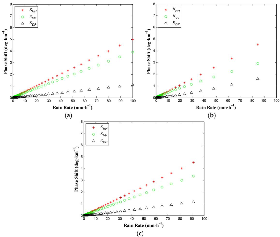
**Figure 5.** Polarimetric propagation parameters vs. rain rate under three different rain types at the L1 (1575.42 MHz) frequency of GPS signals. (a) Stratiform rain; (b) cumuliform rain; (c) mixed clouds rain.
