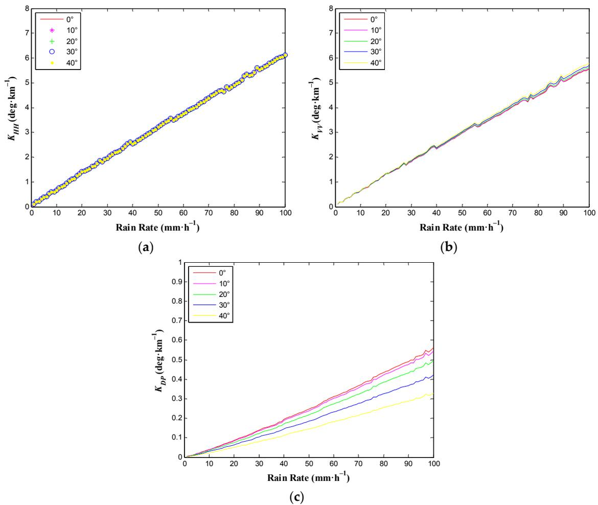
**Figure 4.** Polarimetric propagation parameters vs. rain rate for various elevation angles at the L1 (1575.42 MHz) frequency of GPS signals. (a)  $K_{HH}$ -R; (b)  $K_{VV}$ -R; (c)  $K_{DP}$ -R.
