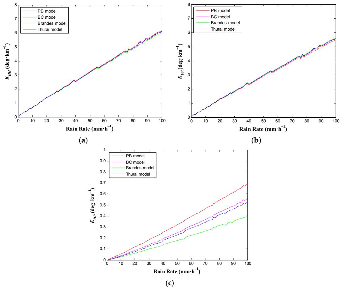
**Figure 2.** Polarimetric propagation parameters vs. rain rate for various shapes of raindrops at the L1 (1575.42 MHz) frequency of GPS signals. (a)  $K_{HH}$ -R; (b)  $K_{VV}$ -R; (c)  $K_{DP}$ -R.
