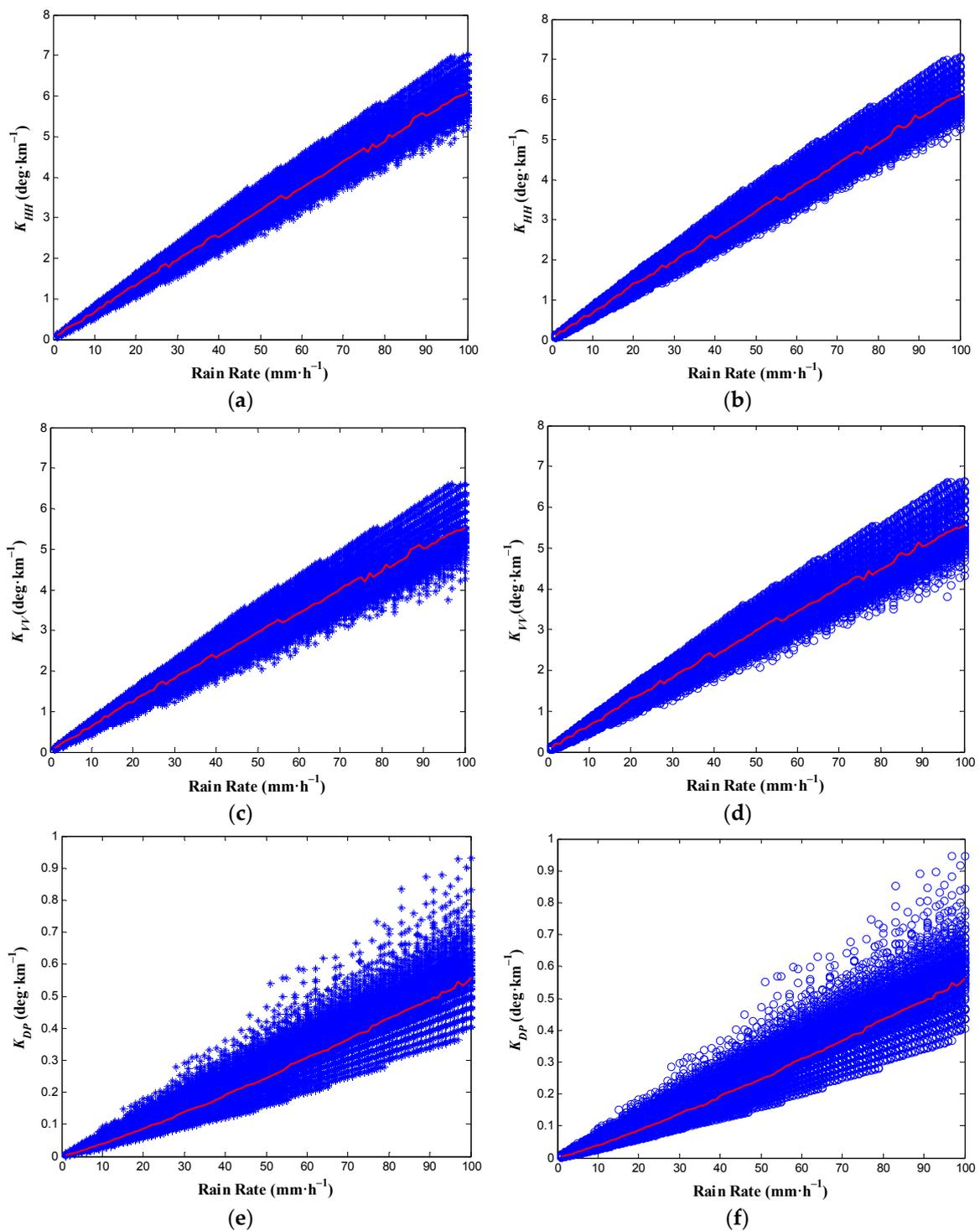
**Figure 1.** Results of polarimetric propagation parameters vs. rain rate at the L1 (1575.42 MHz) frequency of GPS signals based on simulated raindrop size distribution. (a)  $K_{HH}$ -R using Rayleigh Scattering Approximation; (b)  $K_{HH}$ -R using T-matrix; (c)  $K_{VV}$ -R using Rayleigh Scattering Approximation; (d)  $K_{VV}$ -R using T-matrix; (e)  $K_{DP}$ -R using Rayleigh Scattering Approximation; (f)  $K_{DP}$ -R using T-matrix.
