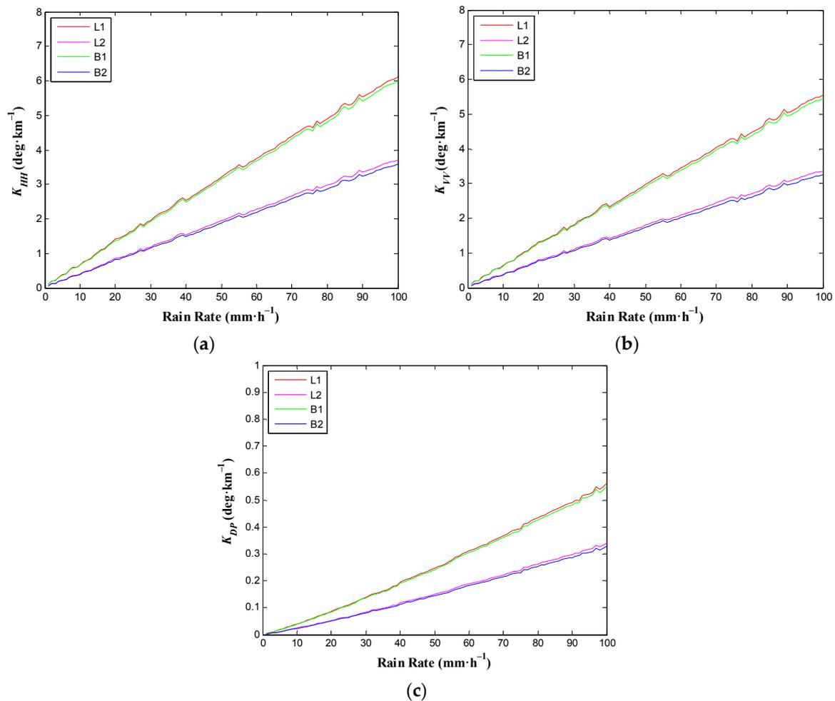
**Figure 3.** Polarimetric propagation parameters vs. rain rate for frequencies of GPS and BeiDou signals. (a)  $K_{HH}$ -R; (b)  $K_{VV}$ -R; (c)  $K_{DP}$ -R.
