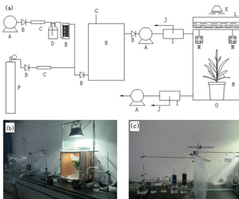
**Figure 1.** Scheme (a) and pictures (b,c) of the experimental apparatus for measuring the removal of aldehyde by plants. (A: pump; B: valve; C: flowmeter; D: Dinitrophenylhydrazine (DNPH)-Acid aqueous solution; E: activated charcoal; F: CO<sub>2</sub> gas; G: aldehydes solution injection port; H: gas mixing bag; I: buffer vessel; J: gas sampling port; K: lamp; L: water tank; M: fan; N: potting-plant; O: exposure chamber. All apparatus were connected by Teflon tubes.)
