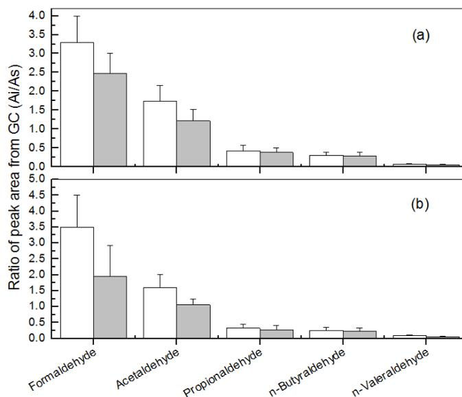
**Figure 4.** The ratios of peak area derived from GC of C<sub>1</sub>–C<sub>5</sub> aldehydes (Ai) to internal standard (As) from the inlet gas (white bars) and the outlet gas (grey bars) of the *Schefflera octophylla* (Lour.) Harms (a) and *Chamaedorea elegans* (Lour.) Harms (b), species enclosed in the chamber at light intensity of about 600 lx respectively. Mean  $\pm$  S.E. are shown.
