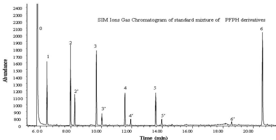
**Figure 2.** SIM Ion: selective ion monitoring ion Gas Chromatograms of standard mixture of Pentafluorophenyl hydrazine (PFPH) derivatives. Peaks 0: PFPH; 1: formaldehyde; 2 and 2': acetaldehyde; 3 and 3': propionaldehyde; 4 and 4': n-butyraldehyde; 5 and 5': valeraldehyde; 6 and 6': 4-fluorobenzaldehyde (IS). The numbers from 2' to 6' are the isomers of the corresponding aldehydes.
