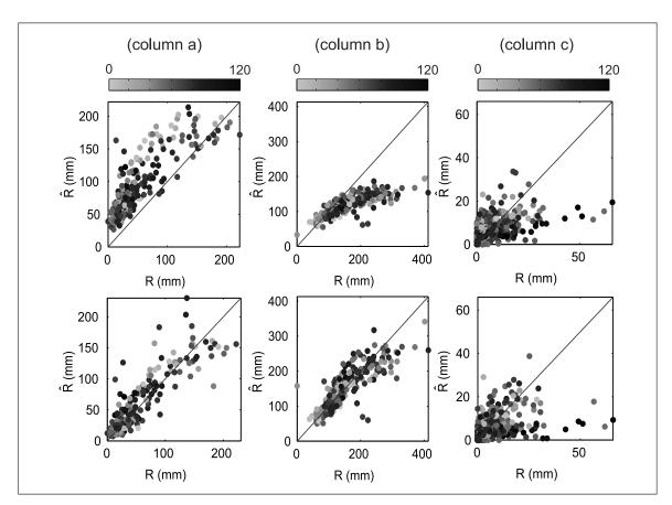
**Figure 6.** Comparison between observed precipitation and rainfall estimated with the regional formula (top graphs) and with the ATS technique (bottom graphs). The comparison is made at the event scale for event 15 (column **a**) and 13 (column **b**). Comparison in (column **c**) refers to event 3 at the hourly scale. (The grey scale refers to the distance from radar, in km).
