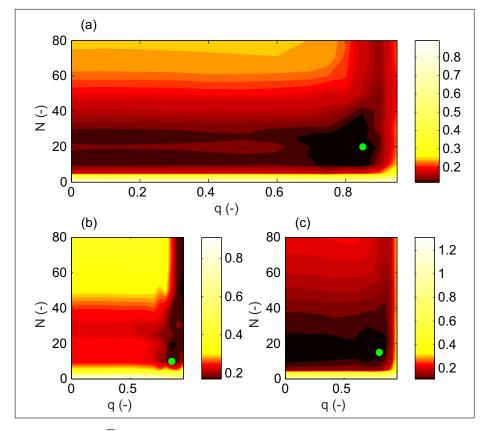
**Figure 4.** Pattern of the  $\overline{I}_3$  index into the parameter space q-N (**a**) for all the selected events, (**b**) for convective only, (**c**) and for stratiform only events. q=0 implies the application of the methodology without any threshold. The green dots indicate the location of the minima.
