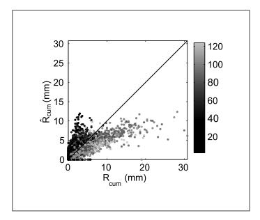
**Figure 3.** Comparison between observed precipitation  $R_{cum}$  and rainfall estimated with the regional formula  $\hat{R}_{cum}$  for the event occurred on 10/31-11/1/2003 at the event scale. (The grey scale refers to rain gauge distance from radar in km).
