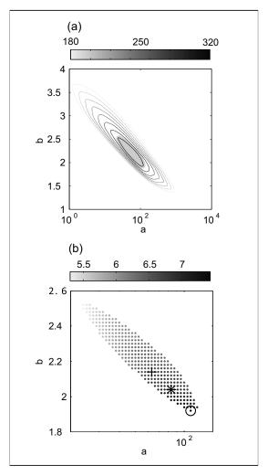
**Figure A1.** (a) Ellipse of the absolute error (greyscale ellipses, mm) into the parameter space a-b. Grey dots represent the sub-minimum area; (b) Values of the *BIAS* (greyscale dots) and location of the minimum of the absolute error (+), of the *BIAS* (o) and of  $I_3$  index (\*) into the sub-minimum space for one of the selected events.
