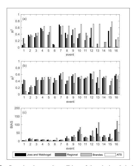
**Figure 5.** Comparison between the coefficients of determination obtained with the Joss-Waldvogel formula, the regional formula, the methodology proposed in [26] and the ATS technique (a) at the event scale and (b) at the hourly scale. Correlation coefficient  $R^2$  falling outside the range (0,1) have not been reported. (c) reports the comparison between the *BIAS* obtained with the four above-mentioned methodologies at the event scale.
