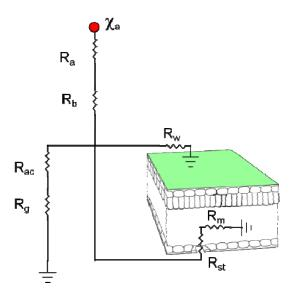
Figure 1. Schematic of dry deposition model for soil and leaf.
