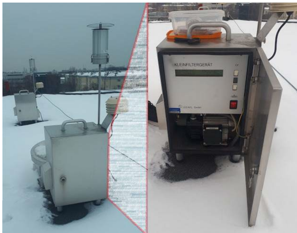
Figure 2. Low-volume sampler LV Leckel; the right-hand side shows an internal exploded view of the main components (Krakow).
