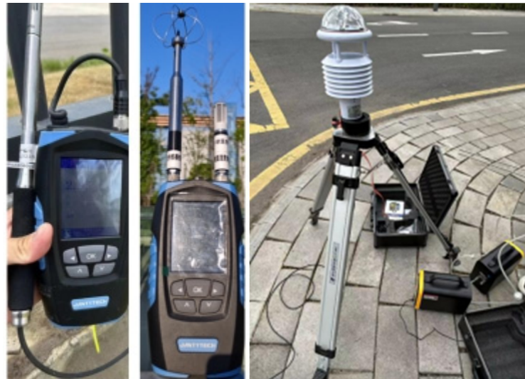
Figure 2. The measuring instruments, from left to right, are the JT2023B wind speed tester, the JT2020 multifunctional tester, and the PC-8(A) mobile weather station.
