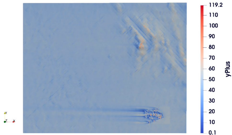
Figure 8. y^+ achieved with the mesh from current work.
