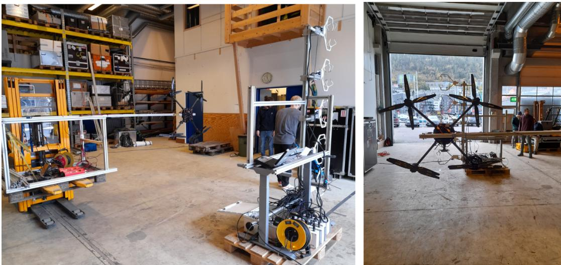
**Figure 3.** Mounting rack for the drone assembled to a forklift and the sonic rig used during the experiment (left panel) and view from behind through the 90° tilted drone towards the bay door that was open during the measurements (right panel).
