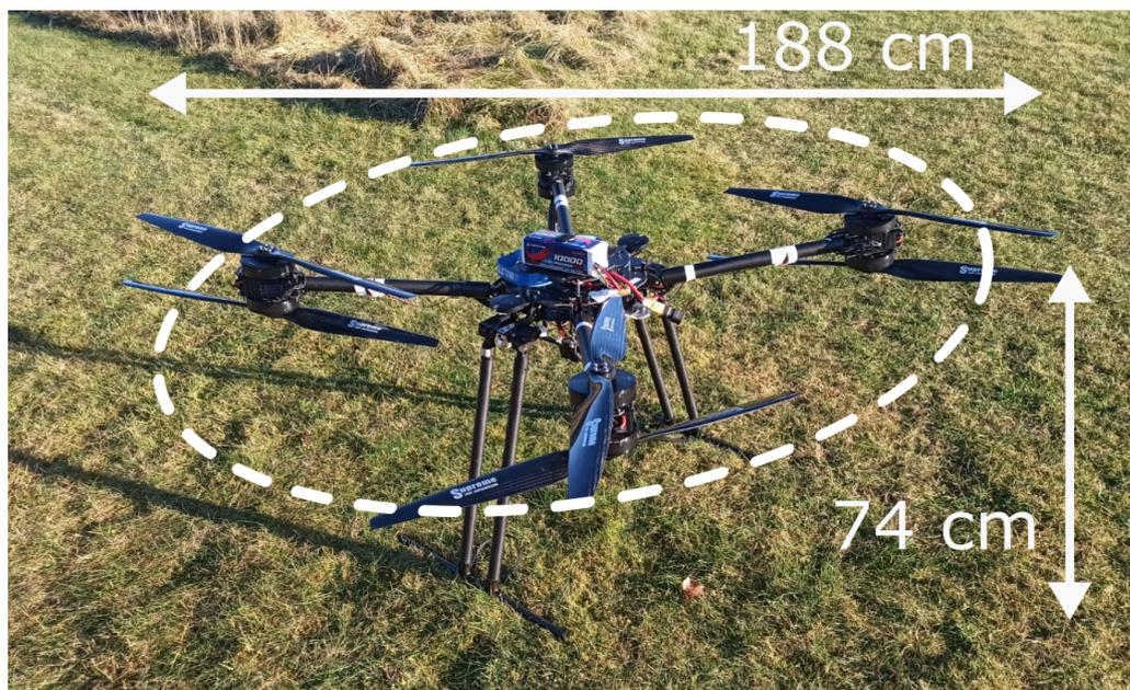
**Figure 1.** Image of the rotary-wing UAV Foxtech D130 X8 and its overall dimensions.
