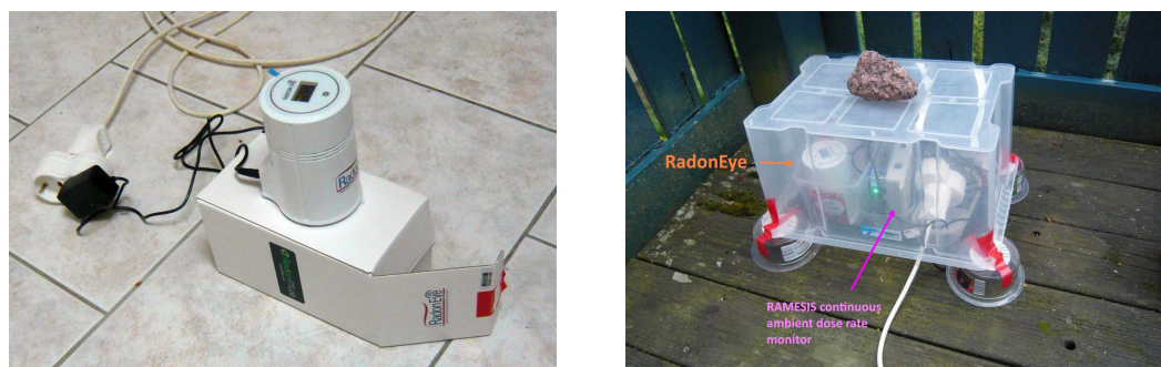
Figure 1. RadonEye, basic model; indoors and outdoors. Parallel ambient dose rate measurements (right picture) are not discussed in this paper. For long-term operation outdoors, an additional protective cover of plastic sheets was applied, and the device was anchored at the balcony grid.
