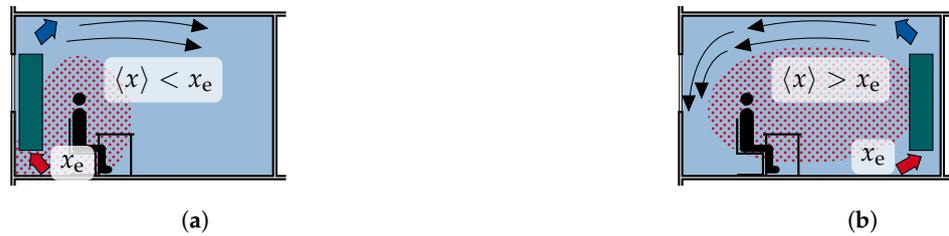
**Figure 8.** Different ranges of the contaminant removal effectiveness for a room equipped with a mobile air purifier in the style of Mundt [55]: (a) contaminant source near the air purifier; (b) contaminant source within the recirculation zone produced by the air purifier.
