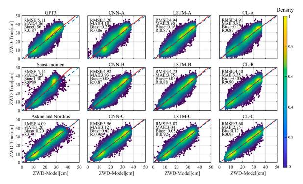
**Figure 10.** Comparison of the forecasting accuracy of the different models in 2022 (The dashed and solid lines represent the theoretical and practical correlation trends between ZWD-Model and ZWD-True, respectively).
