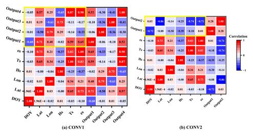
**Figure 9.** The Pearson correlation coefficients between input data and CNN intermediate layer outputs (The yellow box indicates the extraction ability of the CNN intermediate layer to capture important features of the input data). (a) for the first convolutional layer (CONV1); (b) for the second convolutional layer (CONV2).
