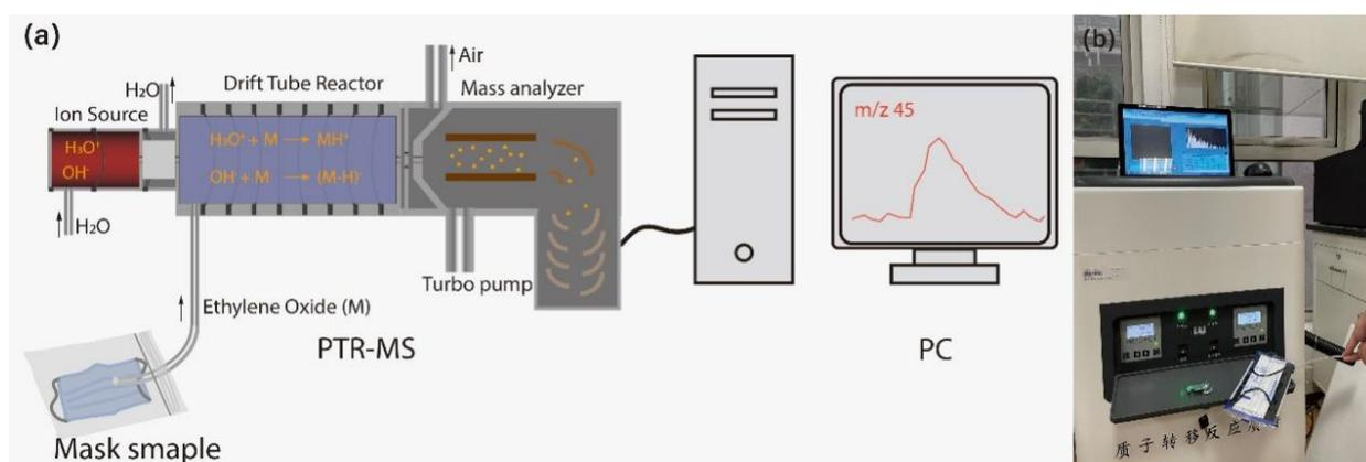
**Figure 1.** (a) Principle of dynamic detection of ethylene oxide concentration in masks using PTR-MS; (b) actual measurement process.
