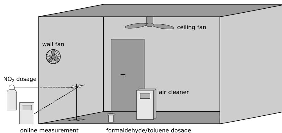
**Figure 1.** Schematic of the CADR test chamber.
