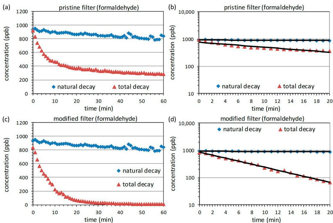
**Figure 2.** Natural (blue) and total (red) decay curves measured with formaldehyde for the pristine (a,b) and modified (c,d) filters. The whole measurement over 60 min is shown in the linear representation on the left side (a,c), whereas the first 20 min used for fitting are shown in the logarithmic representation on the right side (b,d). Black lines are exponential fits to the data points.
