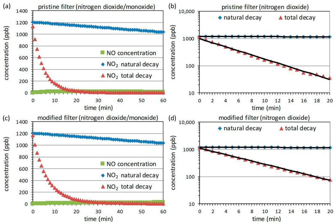
**Figure 4.** Natural (blue) and total (red) decay curves measured with NO<sub>2</sub> for the pristine (a,b) and modified (c,d) filters. Additionally, the measured NO concentration is shown in green for both filters. The whole measurement over 60 min is shown in the linear representation on the left side (a,c), whereas the first 20 min used for fitting are shown in the logarithmic representation on the right side (b,d). Black lines are exponential fits to the data points.
