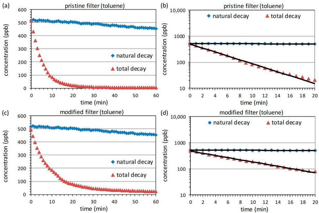
**Figure 3.** Natural (blue) and total (red) decay curves measured with toluene for the pristine (a,b) and modified (c,d) filters. The whole measurement over 60 min is shown in a linear representation on the left side (a,c), whereas the first 20 min used for fitting are shown in a logarithmic representation on the right side (b,d). Black lines are exponential fits to the data points.
