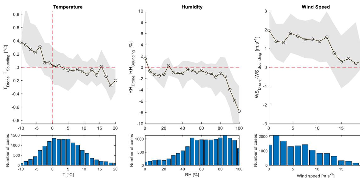
**Figure 7.** Upper panels: the difference between the Meteodrone and radiosonde measurements according to the radiosonde measurements. Left is the temperature, middle is the relative humidity, and right is the wind speed. Black line: median, shaded area: 25–75% percentile. Lower panels: number of observations of each bin.
