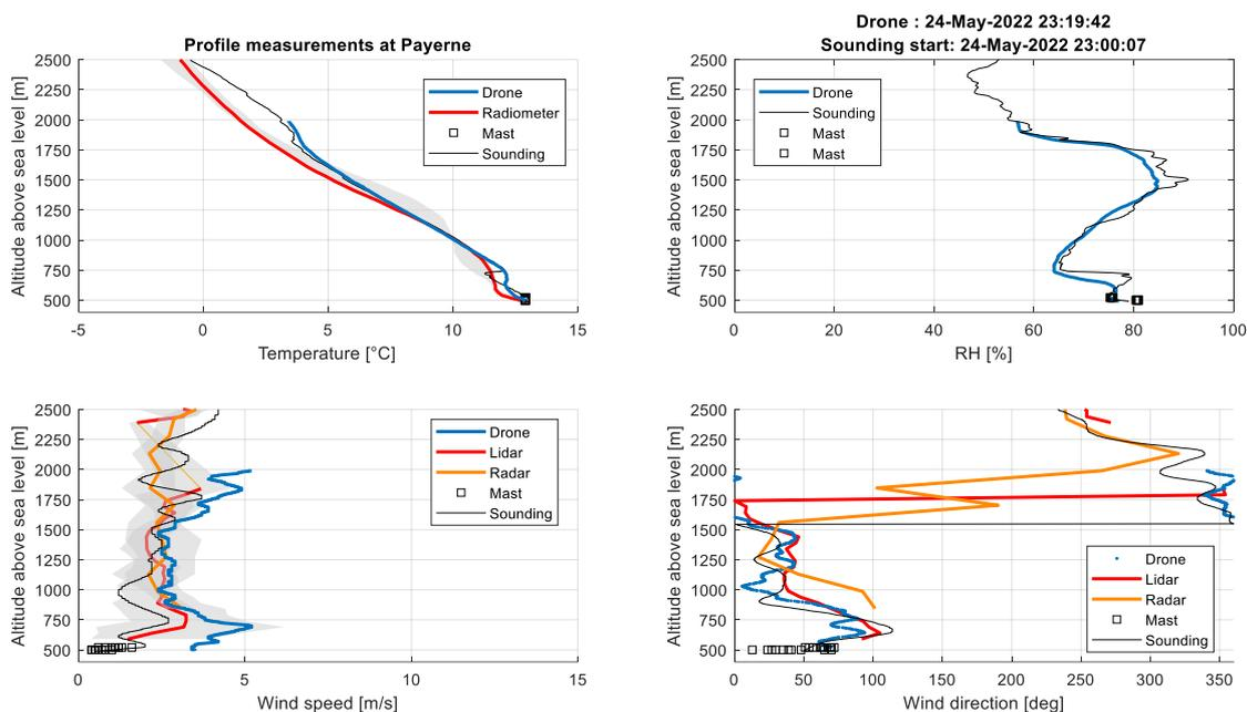
**Figure 4.** Temperature, relative humidity, and the wind speed and direction profiles above Payerne on 24 May 2022 around 23:00 UTC. Drone measurements are in blue, and the radio sounding is in black. The remote sensing measurements are in red, and the radar wind profiler is in orange. The grey areas represent the spread of the remote sensing measurements between 23:00 and 23:30.
