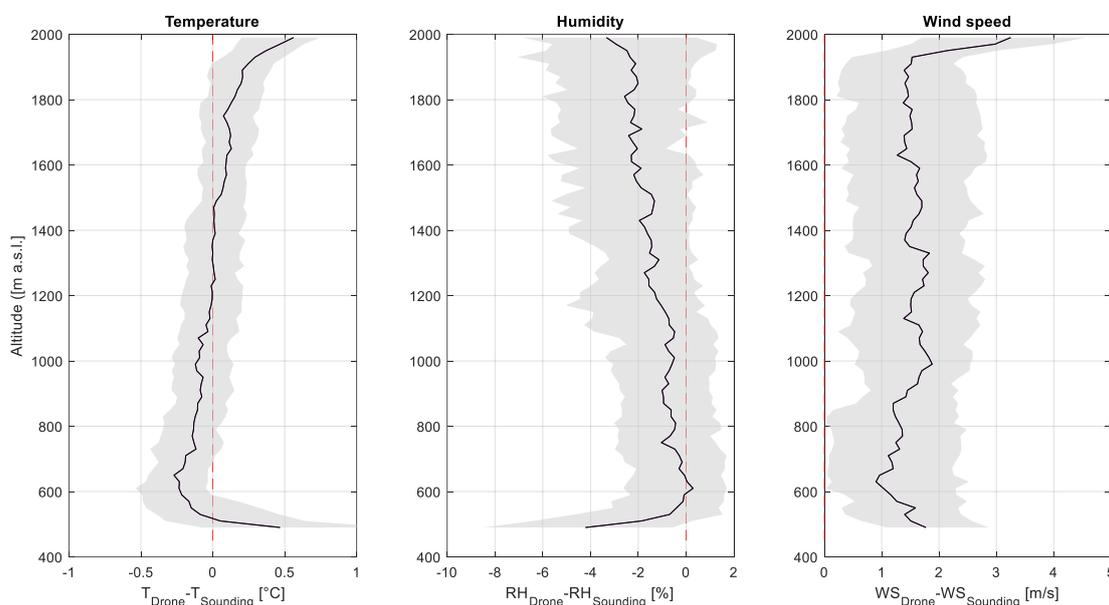
**Figure 6.** Vertical profiles of the difference between the Meteodrone and radiosonde measurements. Left is the temperature, middle is the relative humidity, and right is the wind speed. Black line: median, shaded area: 25–75% percentile.
