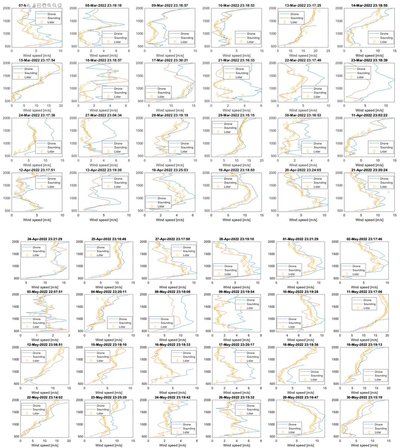
Figure A7. Wind speed profiles measured above Payerne. Blue: Meteodrone, red: radiosounding, and orange: Doppler LiDAR.
