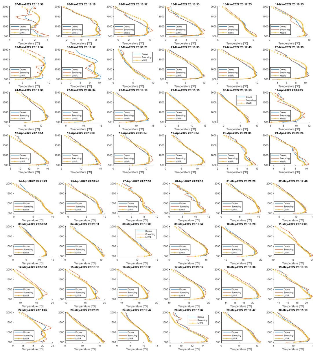
**Figure A5.** Temperature profiles measured above Payerne. Blue: Meteodrone, red: radiosounding, and orange: microwave radiometer.
