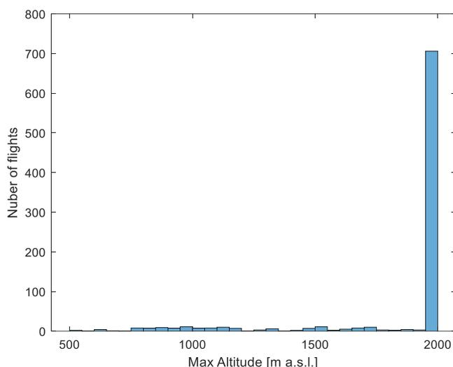
**Figure 3.** Maximum altitude reached by the Meteodrone.
