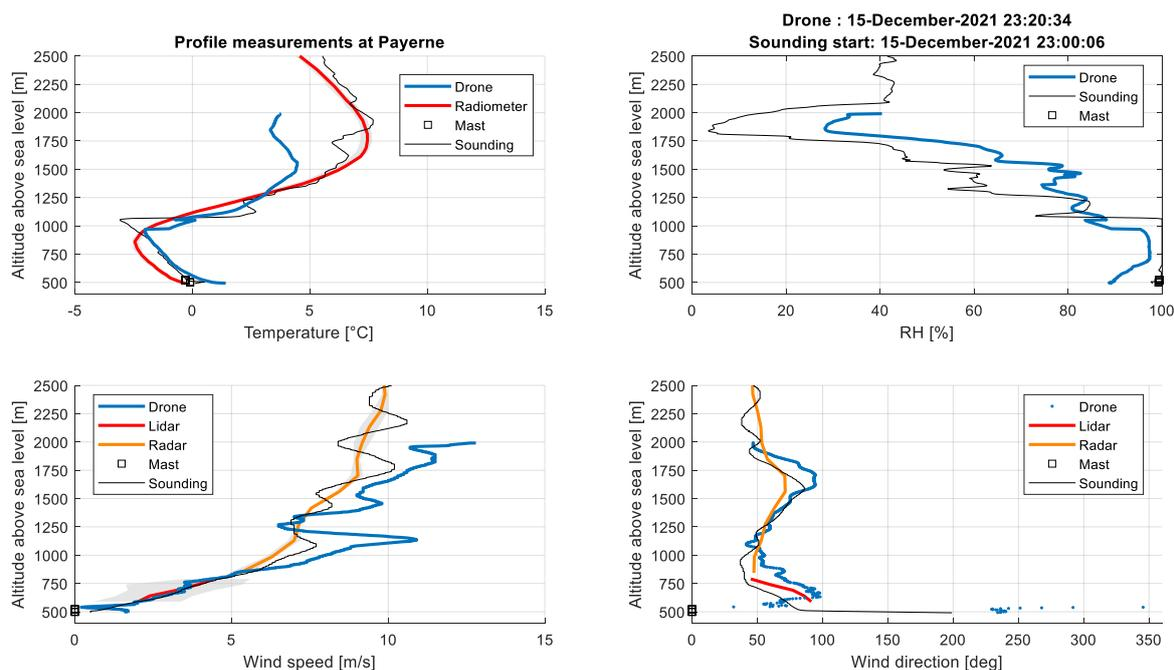
**Figure 5.** Temperature, relative humidity, and the wind speed and direction profiles above Payerne on 15 December 2021 around 23:00 UTC. Drone measurements are in blue, and the radio sounding is in black. The remote sensing measurements are in red, and the radar wind profiler is in orange. The grey areas represent the spread of the remote sensing measurements between 23:00 and 23:30.
