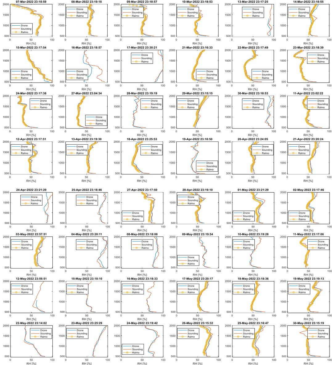
**Figure A6.** Relative humidity profiles measured above Payerne. Blue: Meteodrone, red: radiosounding, and orange: Raman LiDAR RALMO.
