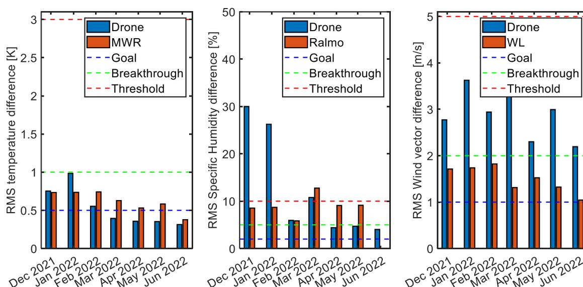
**Figure 8.** Evolution of the RMS of the difference between the radiosondes and Meteodrones (in blue) and remote sensing instruments (in red). Left: temperature, center: specific humidity, right: wind. The WMO requirements for each parameter are represented with dashed lines.
