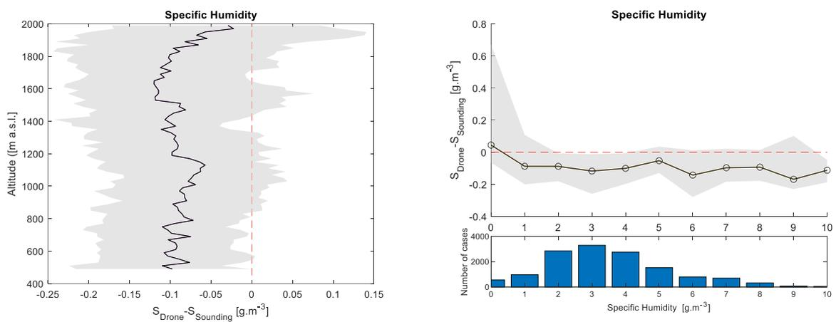
**Figure A10.** Vertical profiles of the specific humidity difference between the Meteodrone and radiosonde measurements(**left**). Difference between the Meteodrone and radiosonde specific humidity measurements according to the radiosonde measurements(**right**). Lower panel: number of observations in each bin. Black line: median, shaded area: 25–75% percentile.
