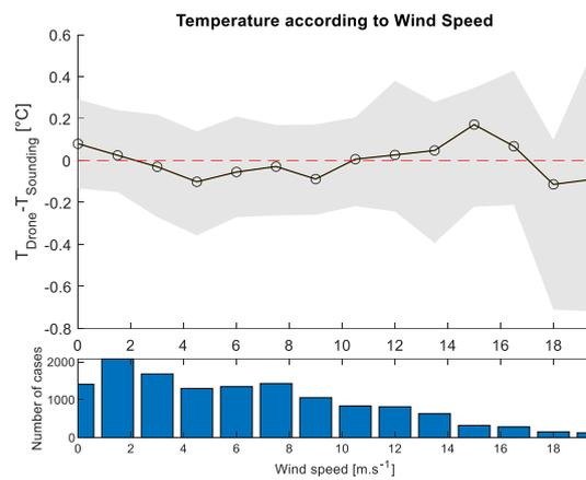
**Figure A9.** Upper panels: Difference between the temperatures measured by the Meteodrone and the radiosonde measurements according to the wind speed measured by the radiosonde. Black line: median, shaded area: 25–75% percentile. Lower panel: number of observations in each bin.
