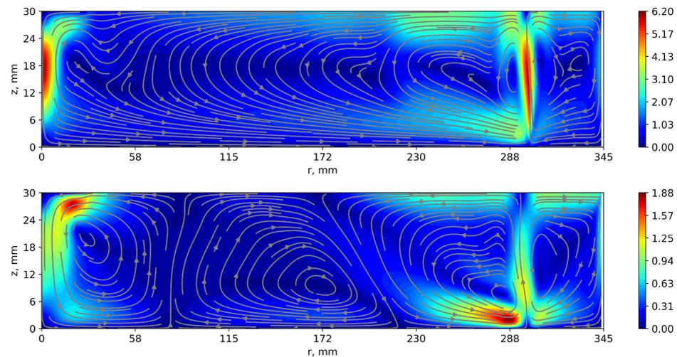
**Figure 9.** Mean meridional circulation for different regimes (averaged over azimuthal coordinate and time). Upper panel – axisymmetric regime (Hadley),  $Ro_T = 8.7$ ,  $Ta = 1.7 \cdot 10^8$ , lower panel— atmospheric-like regime  $Ro_T = 0.4$ ,  $Ta = 3.6 \cdot 10^9$ . Color bar shows magnitude of velocity (in mm/s).
