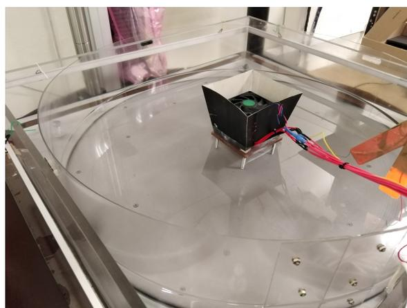
**Figure 2.** (a) Scheme of the laboratory model, 1—rotating table, 2—rim heater, 3—cooler, 4—LED illumination, 5—CCD camera; (b) Photo of the experimental set-up. (Colour online).
