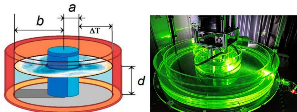
**Figure 1.** Sketch of the BTU experiment (left). Outer (inner) radius  $b(a)$ , fluid height  $d$ , temperature difference  $\Delta T$ . Picture of the annulus taken in the lab (right). See also [27,32].
