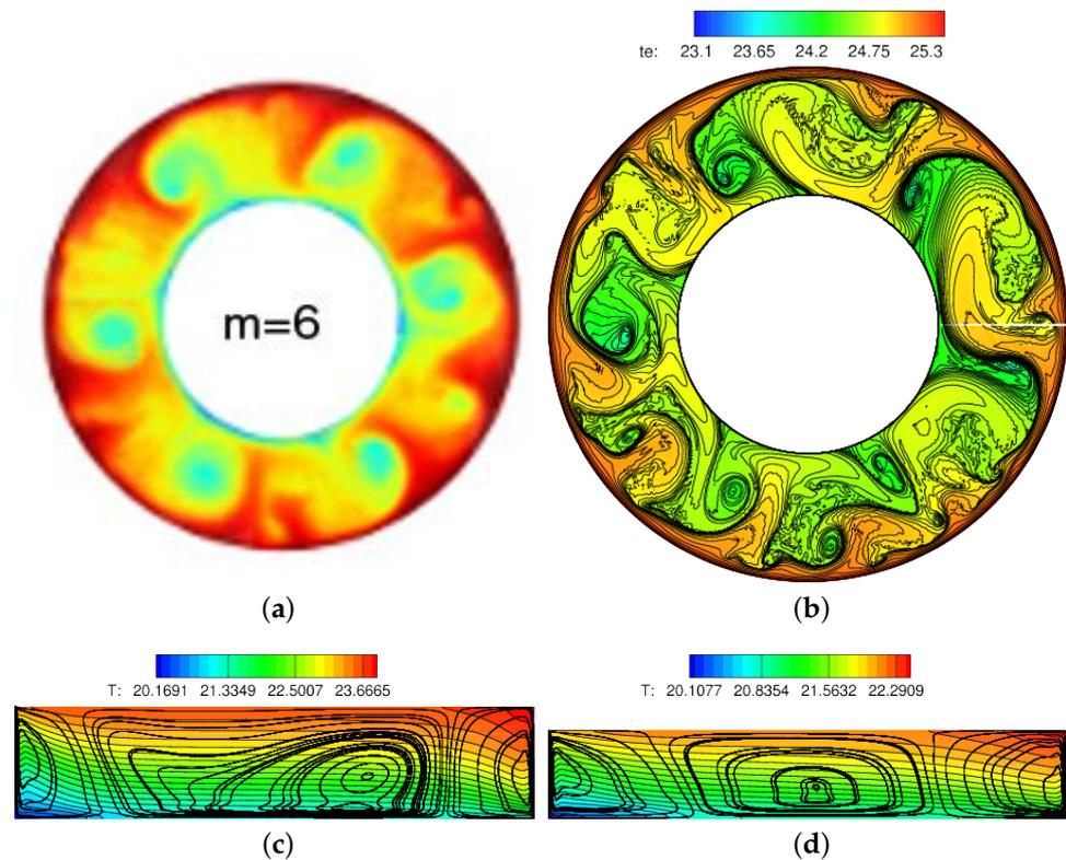
**Figure 4.** Surface temperature measured (a) and simulated for  $\Delta T = 2.5$  K and  $\Omega = 0.7$  rpm (b). Meridional streamfunction derived from the time and azimuthally averaged velocity field from numerical simulations for (c)  $\Delta T = 4$  K and  $\Omega = 2$  rpm, (d)  $\Delta T = 2.5$  K and  $\Omega = 0.7$  rpm.
