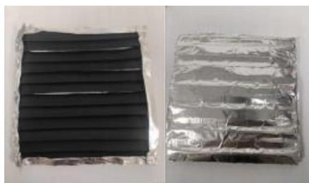
**Figure 1.** Schematic of the wrapped sealing on five sides of the tested material.
