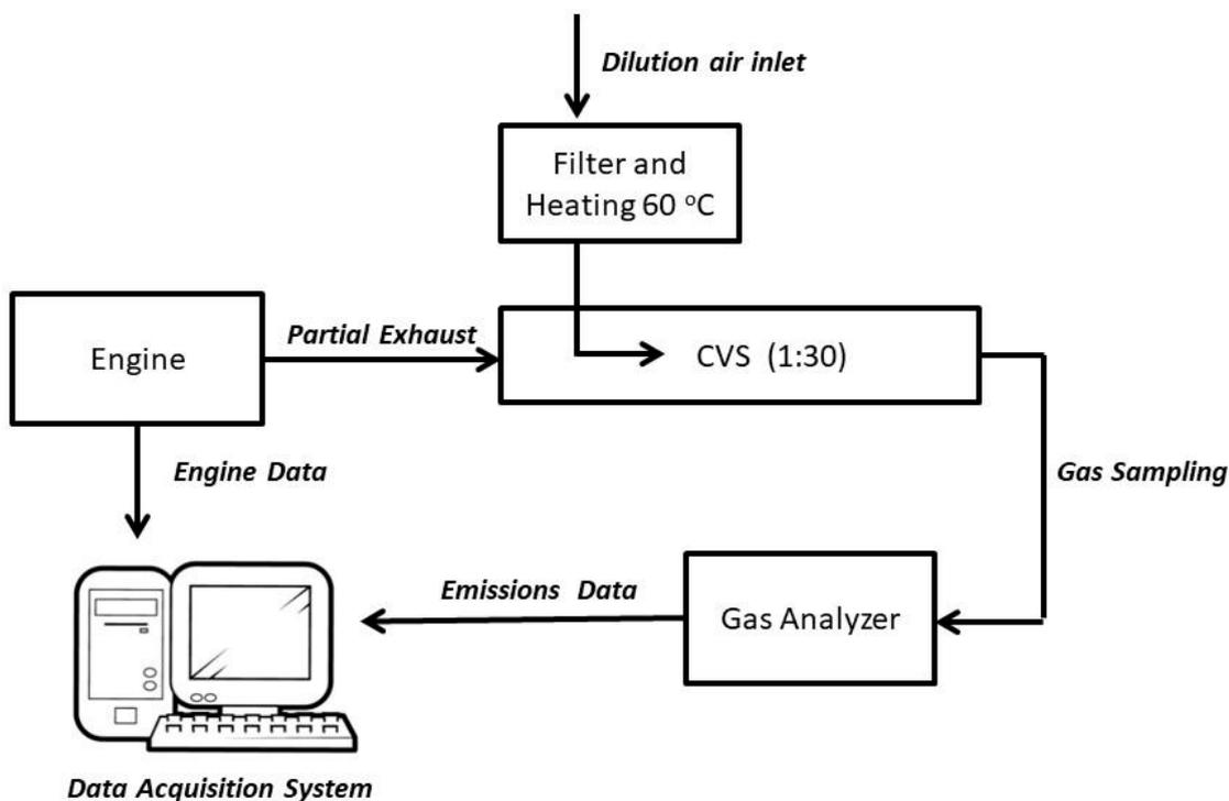
**Figure 1.** Schematic layout of the engine test bed and sampling system for PM<sub>1.0</sub> and PM<sub>2.5</sub>.
