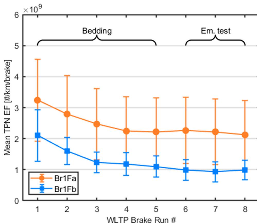
**Figure 8.** Overview of mean TPN emission level for repeated testing of WLTP-Brake cycle for Br1Fa (ECE pad) and Br1Fb (NAO pad) from all labs. The first five runs of the WLTP-Brake cycle correspond to the bedding of the friction pair. Runs 6–8 are the actual emission measurements. The error bars represent the standard deviation from all labs for each run, excluding the volatile particle emission measurements at Lab T for Br1Fa.
