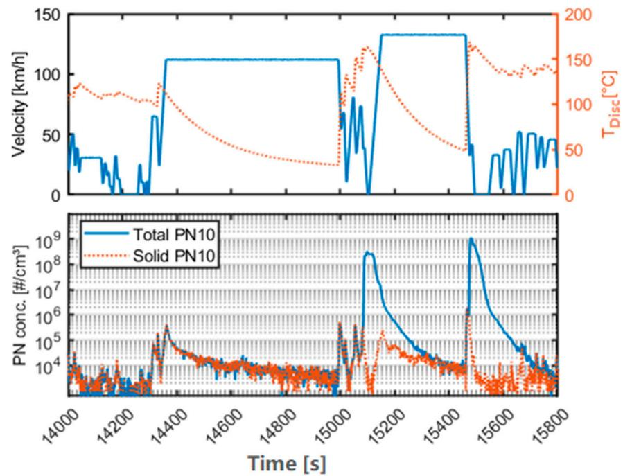
**Figure 6.** Top: velocity and disc temperature. Bottom: total and solid PN concentration during emission run 1 of Lab T for Br1Fa. The TPN emissions increased during high temperature/high speed stops at the end of WLTP Brake Trip 10.
