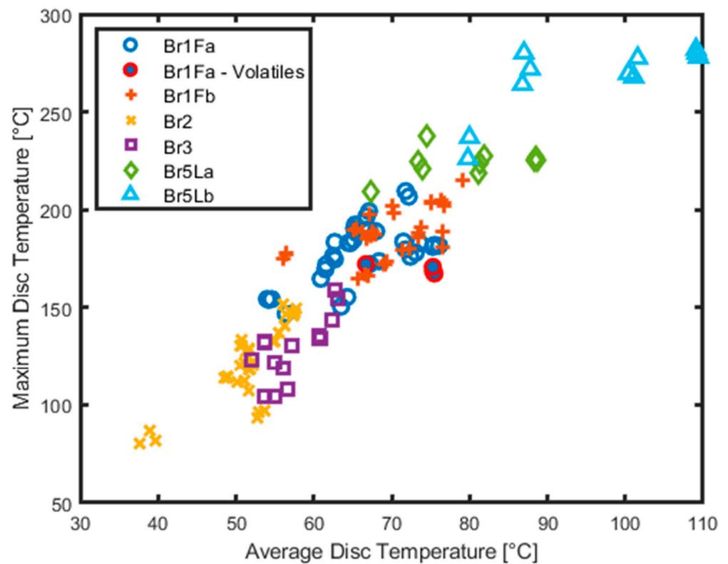
**Figure 7.** Overview of mean and maximum disc temperature for all emission tests. The filled circles highlight measurements with high TPN EF.
