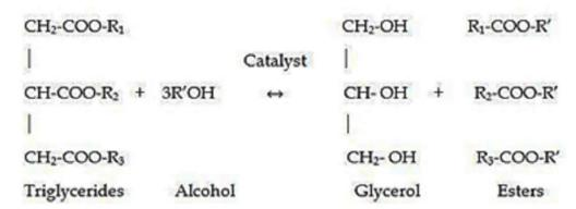
Figure 2. Transesterification reaction.
