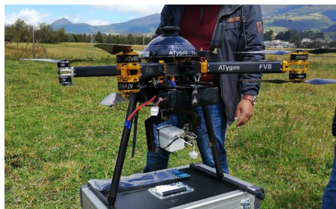
Figure 2. Vaisala RS92-SGP sensor tethered to the ATyges FV8 drone used in this study.
