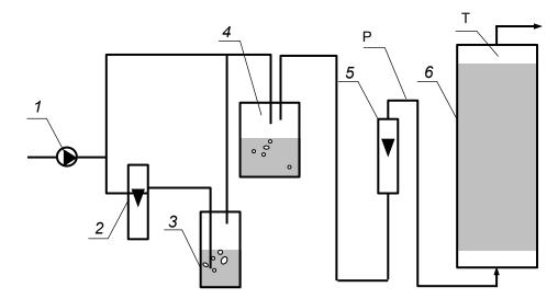
**Figure 1.** Biofilter experimental installation. 1—air pump, 2—rotameter with air valve, 3—bubbler vessel, 4—mixing tank with humidifier (water), 5—rotameter, 6—biofilter, P—sample point of polluted air, T—sample point of treated air.
