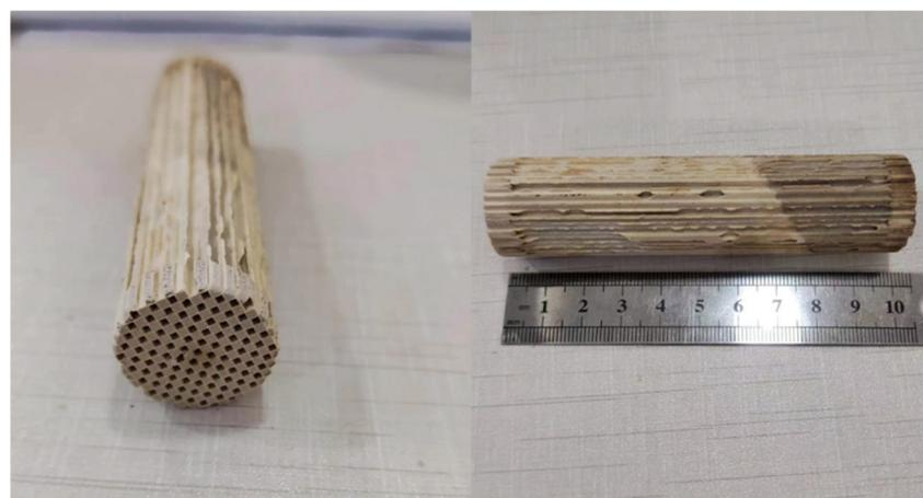
**Figure 2.** GPF test sample.
