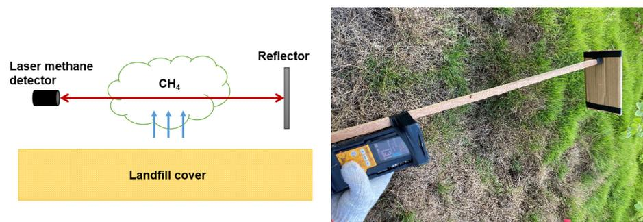
**Figure 3.** Schematic representation of methane concentration measurement using a portable laser methane detector.
