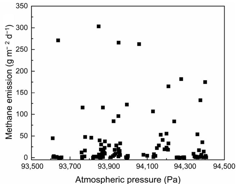
**Figure 6.** Relationship between atmospheric pressure and methane emissions from the landfill cover.
