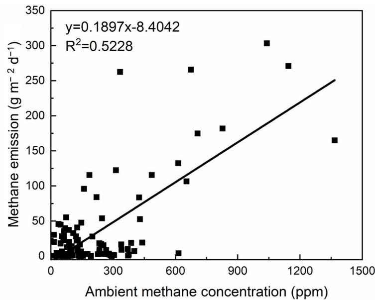
**Figure 8.** Relationship between the measured ambient methane concentrations and methane emissions.
