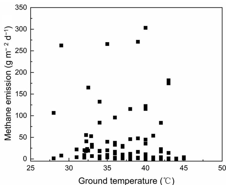
**Figure 7.** Relationship between the measured ground temperature and methane emissions.
