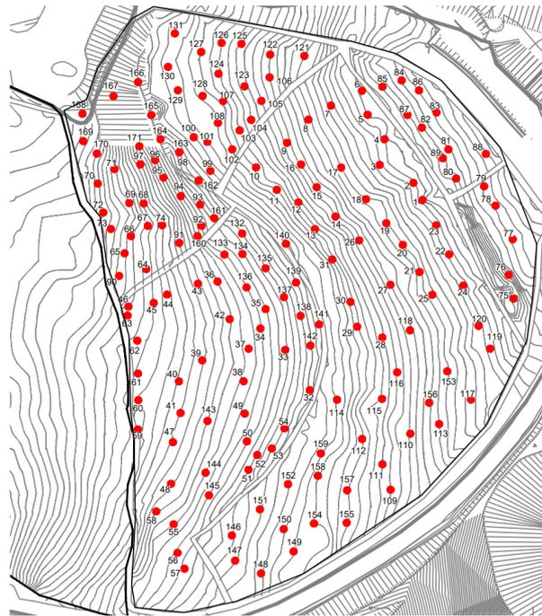
**Figure 2.** Distribution of monitoring points for surface methane concentration in the test area.
