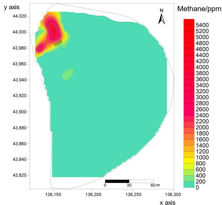
**Figure 5.** Distribution of methane concentrations in the test area measured after rainfall.
