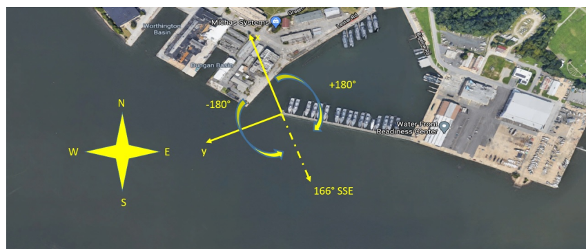
Figure 3. Sensor orientation and wind velocity angle readings compared to compass rose.
