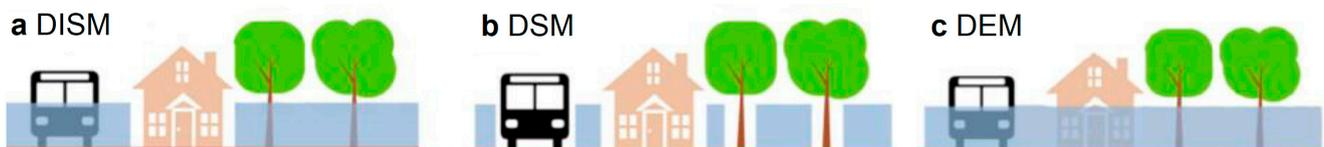
**Figure 7.** Graphical illustration of the differences between (a) DISM, (b) DSM and (c) DEM.
