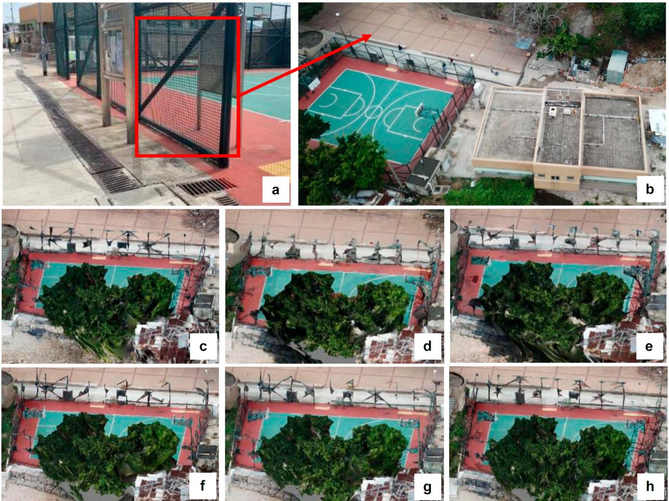
**Figure 6.** Texture analysis of a playground. (a,b) The ground-based view and the UAV aerial photo of the playground. (c–h) The fences of the playground generated under six scenarios.
