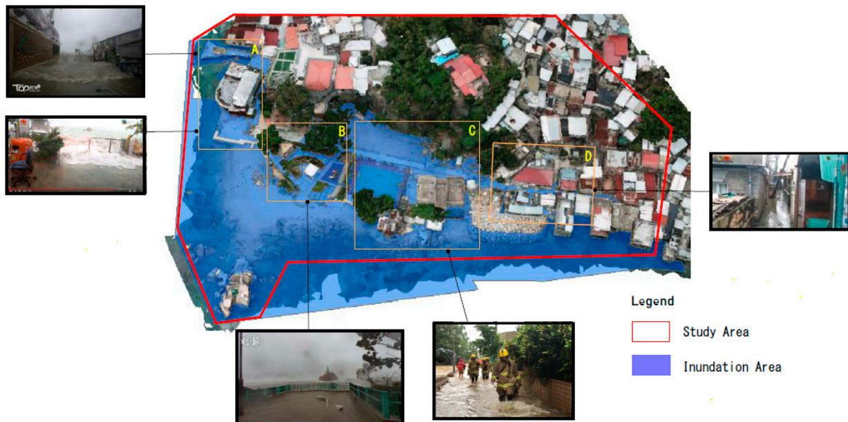
**Figure 14.** Maximum flood area simulated by the DISM under the Typhoon Mangkhut scenario.
