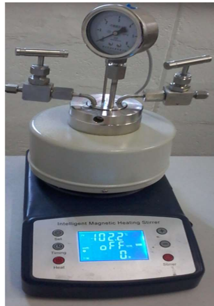
Figure 3. The hydrothermal carbonization reactor.
