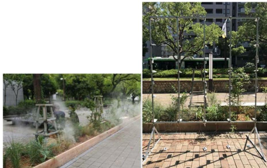
**Figure 4.** Mist spraying and measurement frame in an open space.
