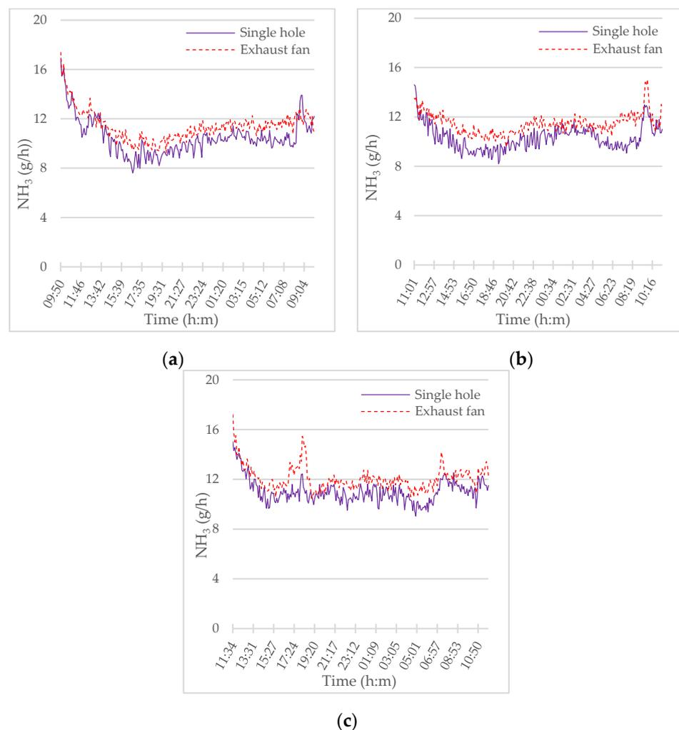
**Figure 5.** The ammonia ( $\text{NH}_3$ ) reduction effect by spraying water inside of the curtain at the maximum operating rate of the barn exhaust fan (100%), (a) S/P (spray time, min./pause time, min.) 10/30, (b) 10/10, (c) 10/5.
