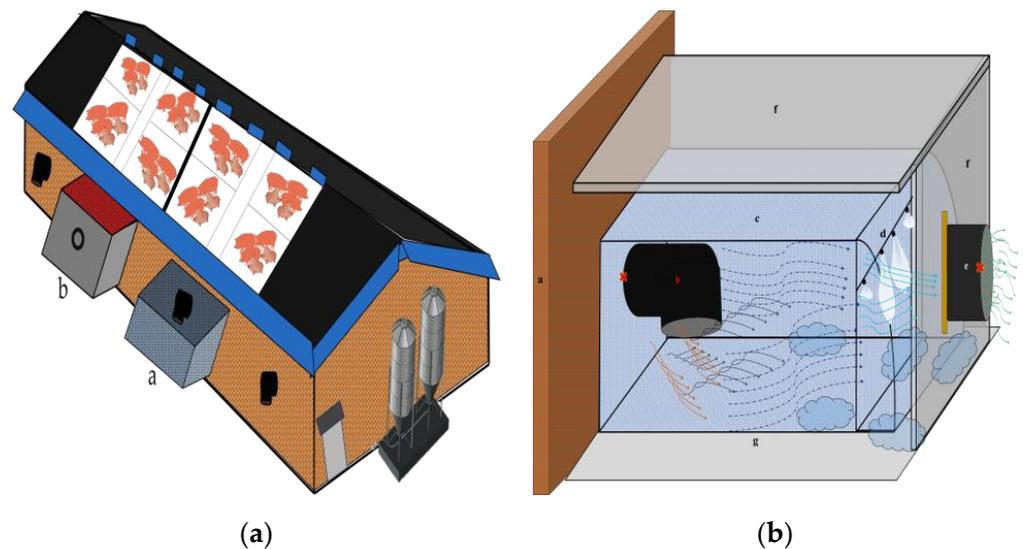
**Figure 1.** Schematic diagram of the experimental setup, (a) swine facility: a. curtain set up, b. metallic cover setup, (b) curtain and metallic cover setup: a. barn wall, b. exhaust fan, c. curtain, d. spraying nozzles, e. single hole, f. metallic cover, g. floor, “x” markings represent the  $\text{NH}_3$  sampling point.
