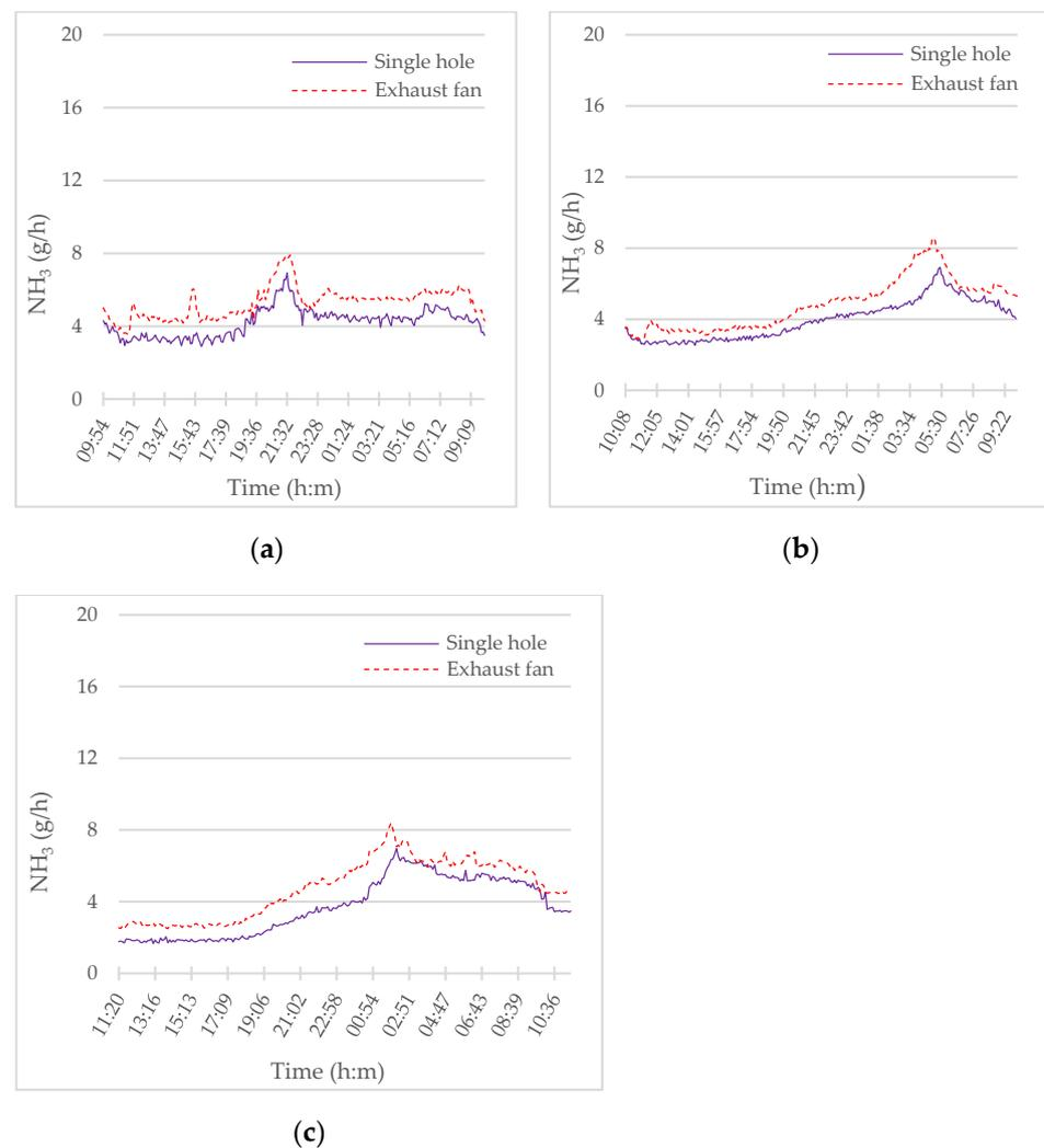
**Figure 7.** The ammonia ( $\text{NH}_3$ ) emission reduction effect by spraying inside the curtain at the minimum operating rate of the barn exhaust fan (30%). (a) S/P (spray time, min./pause time, min.) 10/30, (b) S/P 10/10, (c) S/P 10/5.
