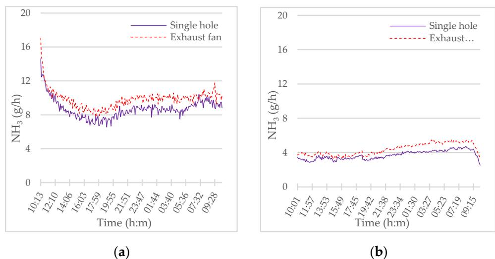
Figure 4. The ammonia (NH<sub>3</sub>) reduction effect in non-spray conditions inside the curtain: (a) the maximum operating rate of the barn exhaust fan (100%), (b) minimum operating rate of barn exhaust fan (30%).
