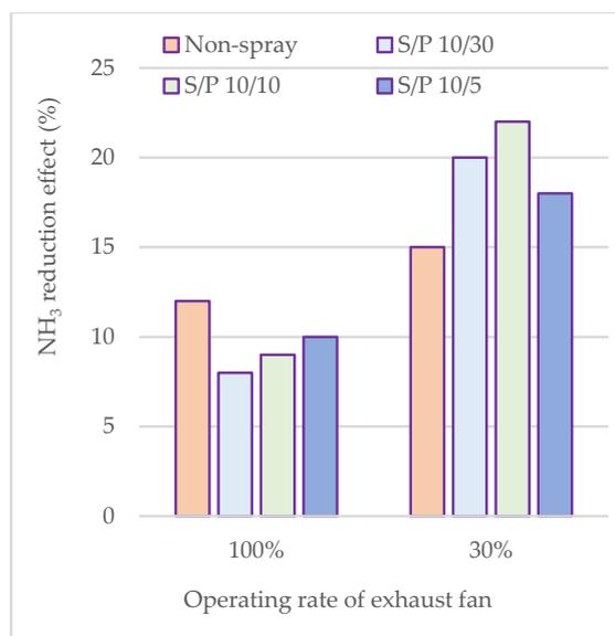
**Figure 6.** The ammonia (NH<sub>3</sub>) reduction effects (%) of non-spraying and spraying water treatment. S/P (spray time, min./pause time, min.) 10/30, S/P 10/10, and S/P 10/5 at the 100% or 30% in operating rate of the barn exhaust fan.
