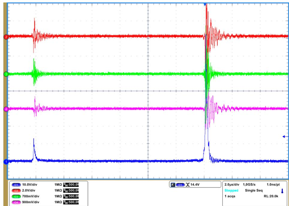
**Figure 11.** Characteristic oscillogram of the first and repeated discharge current pulse (blue signal) from the system of artificial thunderstorm cells of positive polarity with the participation of lower and upper groups of model hydrometeors and signals, registered by antennas A1–A3 (red, green and magenta signals resp.).
