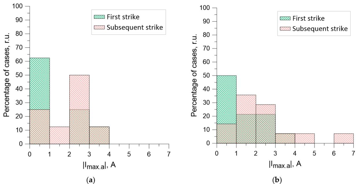
**Figure 15.** Distribution of signal amplitude values of  $I_{\max,a}$ , induced at the antenna A3 by the first and repeated discharges: (a)—variant in Figure 2c; (b)—variant in Figure 2d.
