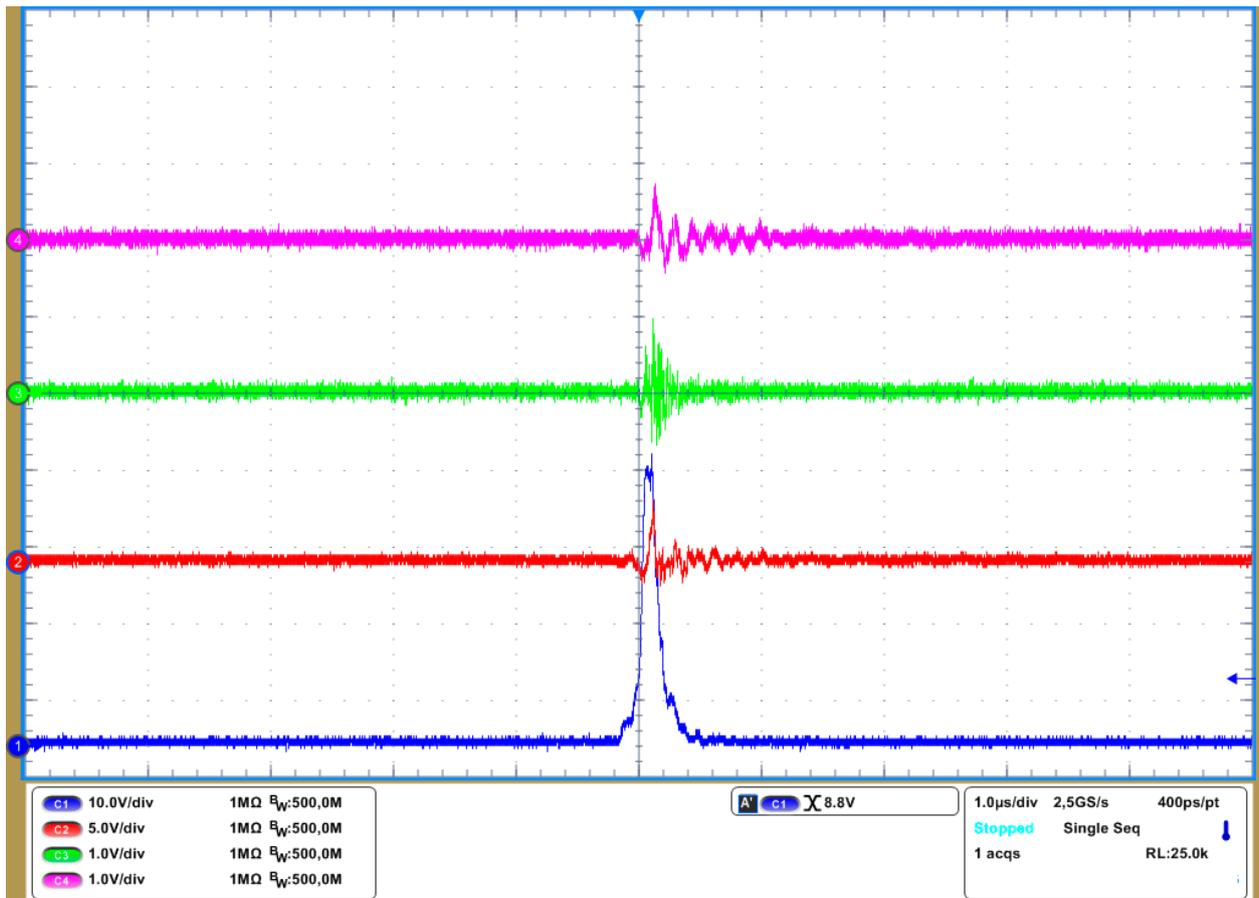
**Figure 4.** Characteristic oscillogram of the main stage discharge current pulse (blue signal) between a single artificial positively charged thundercloud cell and the ground involving one group of model hydrometeors and signals, registered by antennas A1–A3 (red, green and magenta signals resp.).
