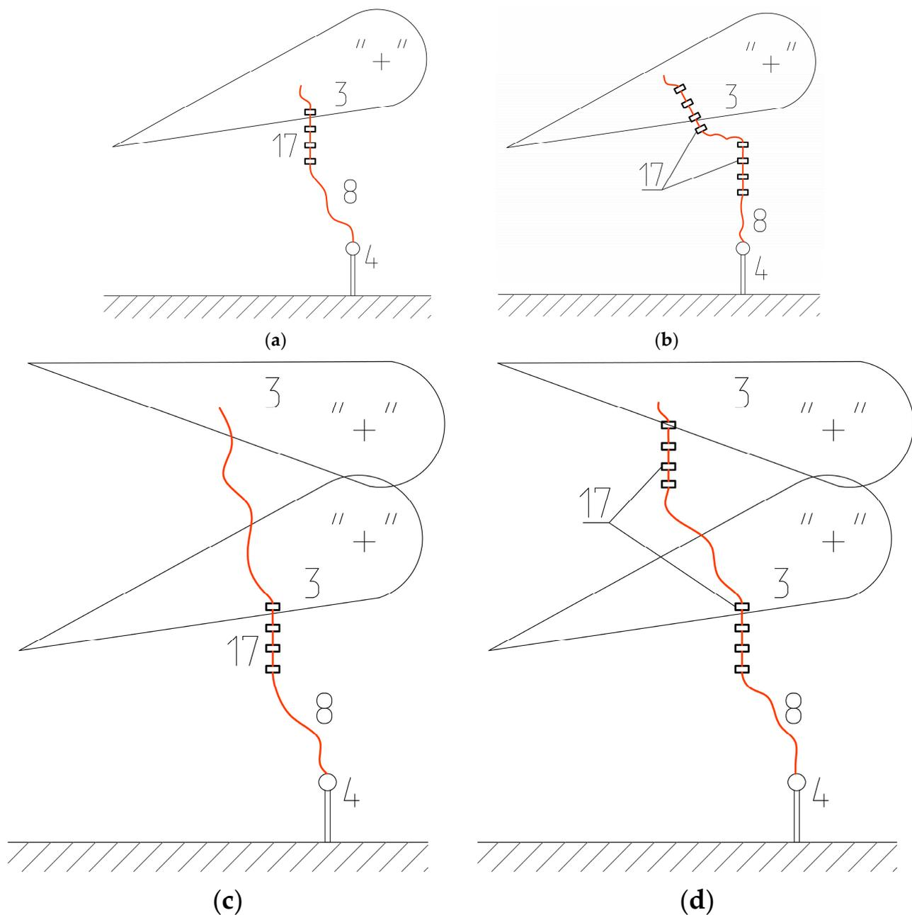
**Figure 2.** Variants of experimental study series with different numbers of artificial thunderstorm cells of positive polarity and model hydrometeor groups (and their arrangement): one artificial thunderstorm cell and one hydrometeor group (a); one artificial thunderstorm cell and two hydrometeor groups (b); two artificial thunderstorm cells and one hydrometeor group (c); two artificial thunderstorm cells and two hydrometeor groups (d).
