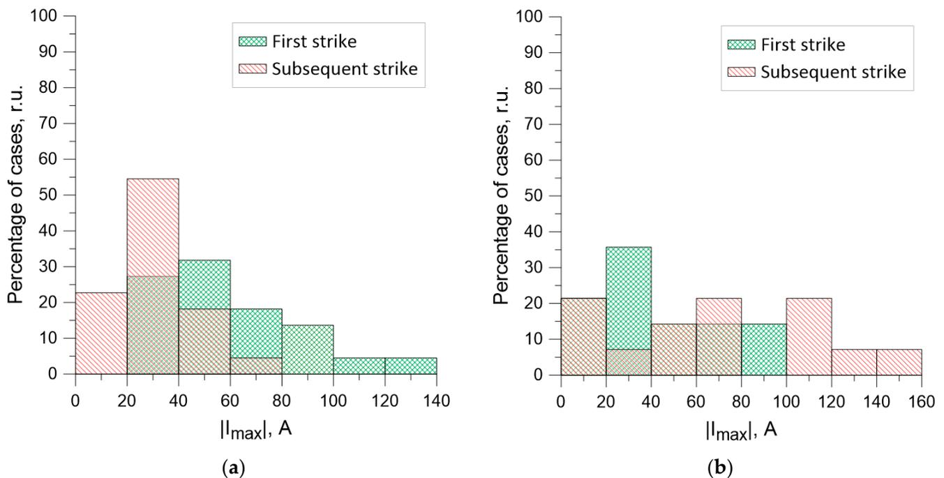
**Figure 14.** Distribution of current pulse amplitude values of the first and repeated discharges at negative polarity of artificial thunderstorm cells (a) and at positive polarity of artificial thunderstorm cells (b).
