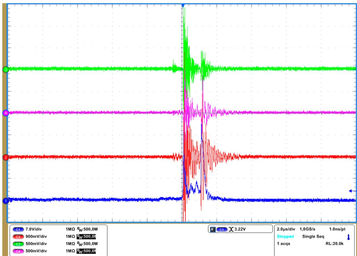
**Figure 6.** Characteristic oscillogram of the first and repeated discharge current pulses (blue signal) between a single artificial positively charged thundercloud cell and the ground involving two groups of model hydrometeors and signals, registered by antennas A1–A3 (red, green and magenta signals resp.).
