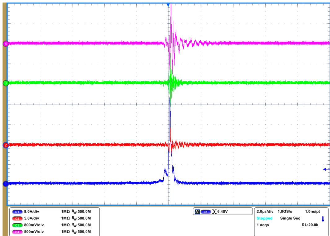
**Figure 10.** Characteristic oscillogram of the current pulse (blue signal) of the main discharge stage with participation of only the lower group of model hydrometeors and signals, registered by antennas A1–A3 (red, green and magenta signals resp.).
