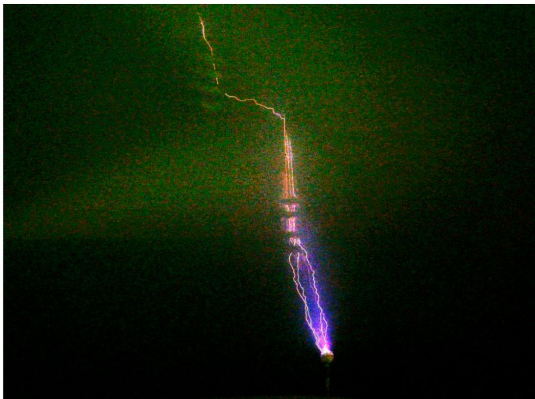
**Figure 9.** Discharge formation between the system of artificial positively charged thunderstorm cells and the ground involving the lower and upper groups of model hydrometeors.
