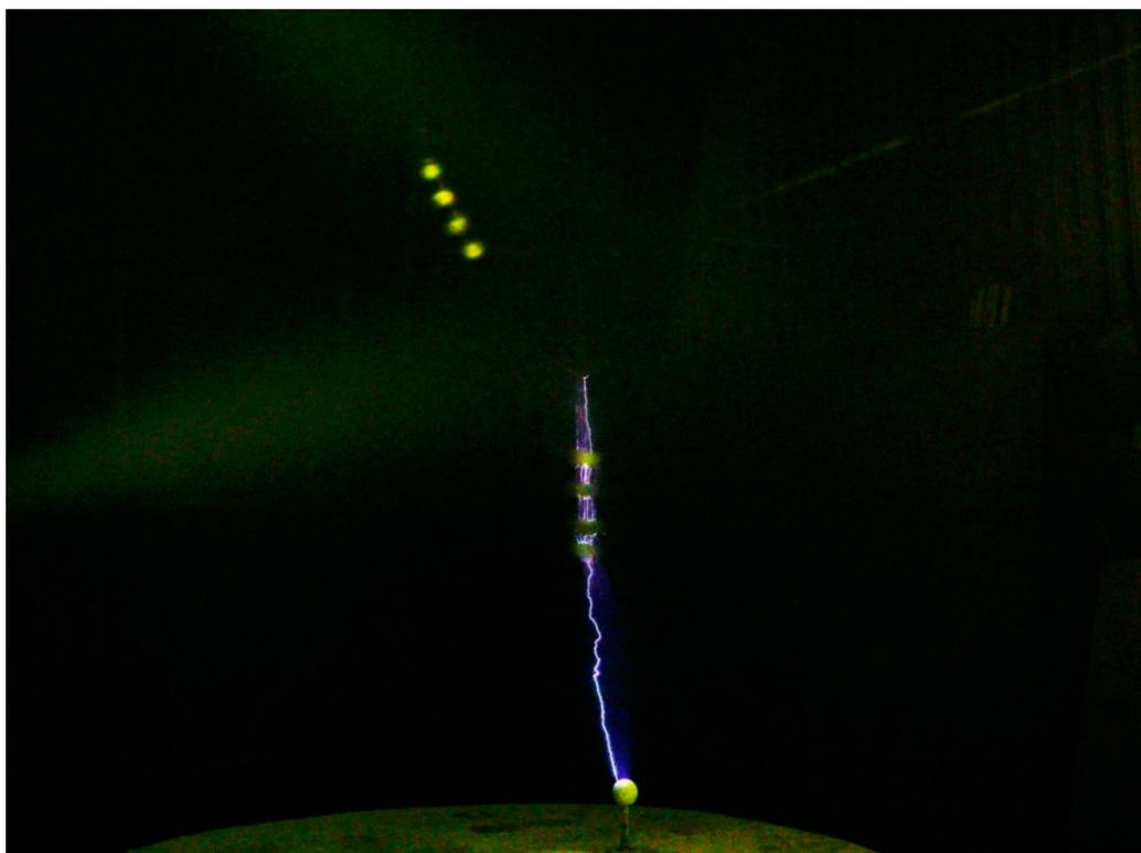
**Figure 8.** Discharge formation between the system of artificial positively charged thunderstorm cells and the ground involving only the lower group of model hydrometeors.
