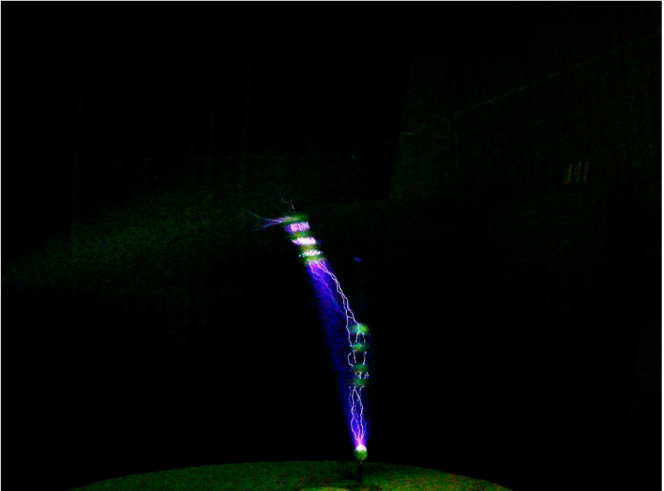
**Figure 5.** Discharge formation between a single artificial positively charged thunderstorm cell and the ground involving two groups of model hydrometeors.
