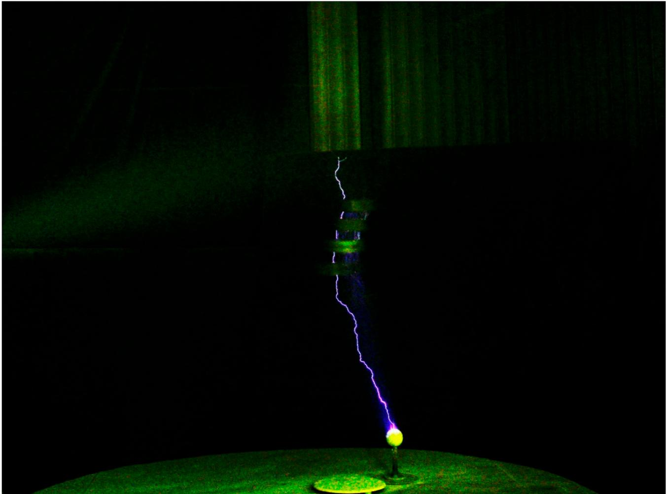
**Figure 3.** Discharge formation between a single positively charged thunderstorm cell and the ground involving one group of model hydrometeors.
