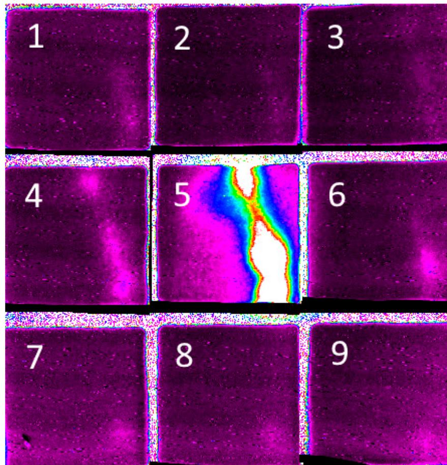
**Figure 7.** Characteristic dynamics of single discharge formation from an artificial thunderstorm cell of positive polarity with the participation of lower and upper groups of model hydrometeors (frame size 75 × 75 cm, frame duration 1.5 μs, pause between frames 0.1 μs).
