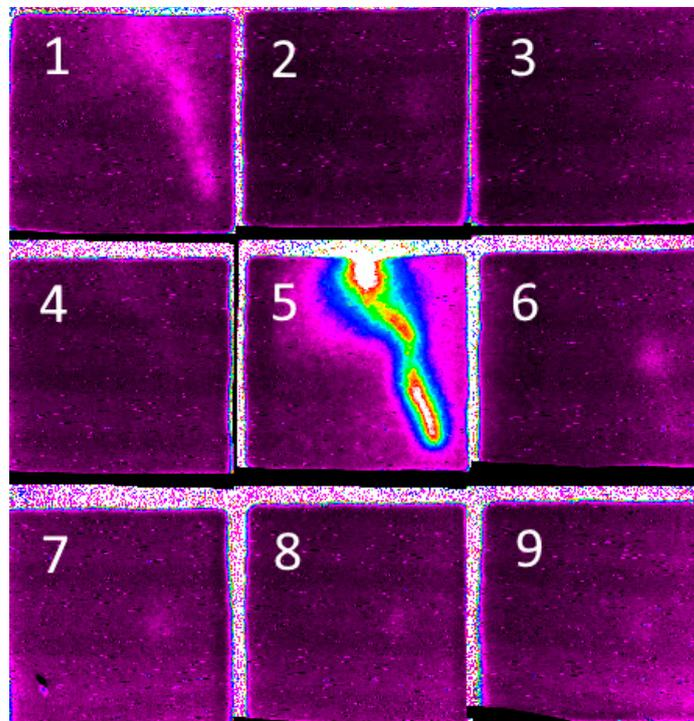
**Figure 12.** Characteristic dynamics of the formation of the first and repeated discharges from the system of artificial thunderstorm cells of positive polarity with participation of lower and upper groups of model hydrometeors at a more powerful repeated discharge (frame size  $85 \times 85$  cm, frame duration  $2.5 \mu\text{s}$ , pause between frames  $0.1 \mu\text{s}$ ).
