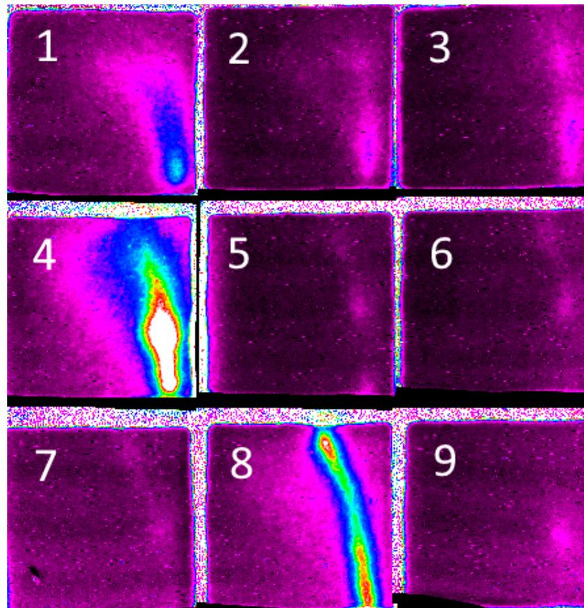
**Figure 13.** Characteristic dynamics of formation of the first and repeated discharge from the system of artificial thunderstorm cells of positive polarity with the participation of lower and upper groups of model hydrometeors at a more powerful first discharge (frame size  $85 \times 85$  cm, frame duration  $2.5 \mu\text{s}$ , pause  $0.1 \mu\text{s}$ ).
