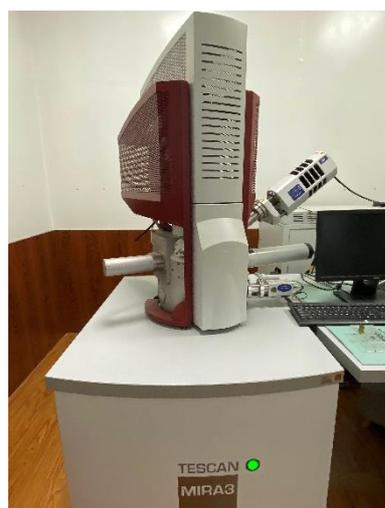
**Figure 1.** MIRA3 field emission scanning electron microscope.
