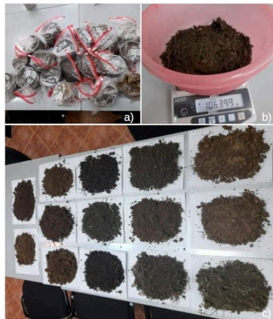
**Figure 3.** Dry soil measurement: (a)—soil sample; (b)—weight measurement; (c)—dry sample.
