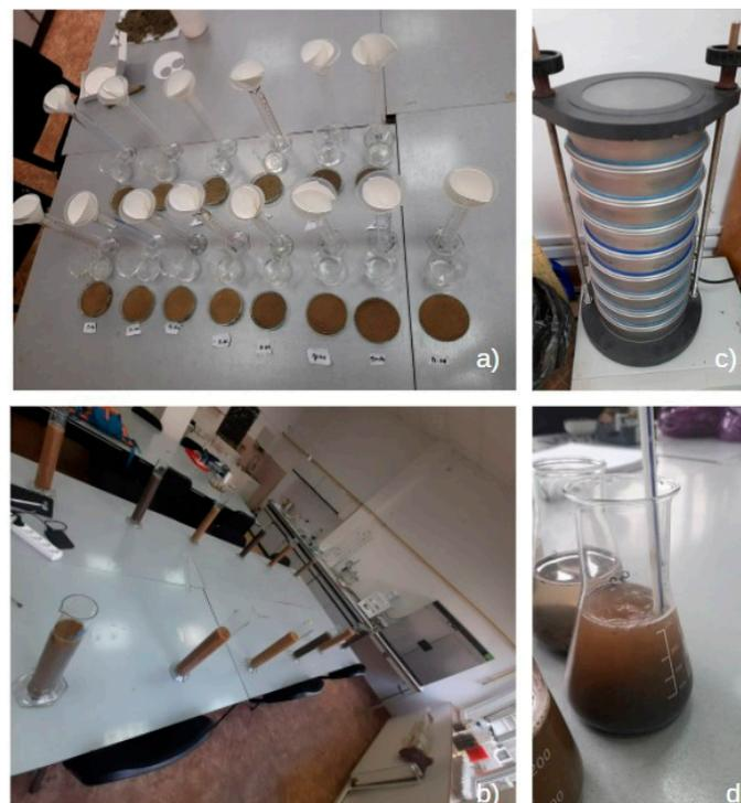
**Figure 4.** Soil properties measurement: (a)—water holding capacity; (b,c)—soil texture; (d)—physico-chemical properties.
