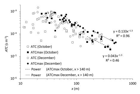
**Figure 4.** Atmospheric transfer coefficients ATC measured at a height of 0.15 as a function of distance x from the discharge point.
