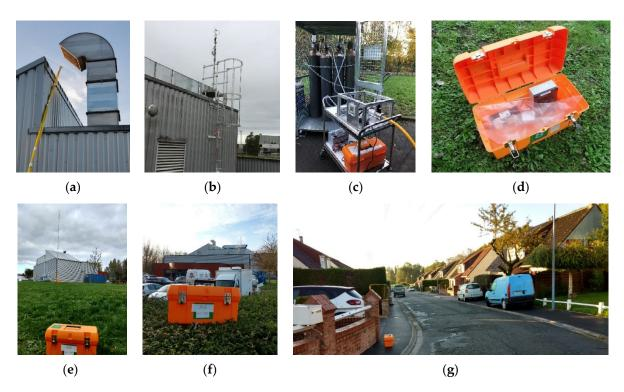
**Figure 2.** (a) Cyclotron discharge stack; (b) Young ultrasonic anemometer on the cyclotron roof; (c) helium discharge system; (d) Atmospheric sampler AS equipped with a sampling pump connected to a Tedlar bag and a flowmeter; (e–g) examples of AS locations at 40 m (e,f) and 150 m (g) from the discharge point.
