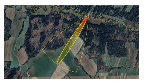
**Figure 12.** Graphical representation of the dispersion of a dangerous substance at the Trstená-Chyžné border crossing [24,25].
