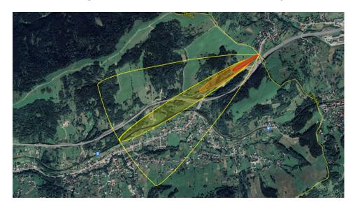
**Figure 7.** Graphical representation of the dispersion of a dangerous substance at the Skalité-Zwardoň-Myto 2 border crossing [24,25].
