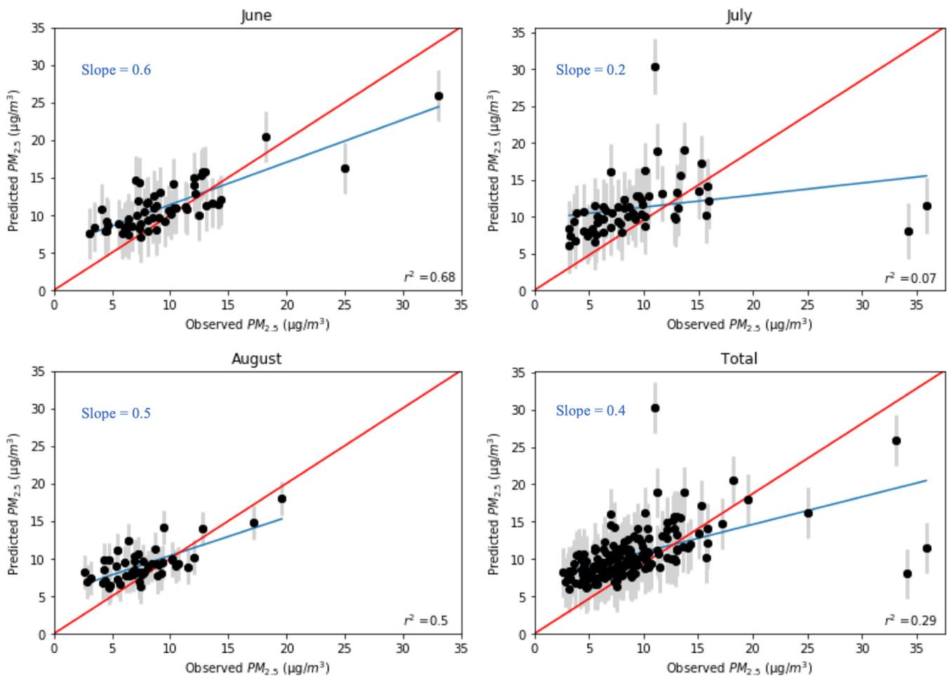
**Figure 7.** Scatter plots for New Hanover County indicating model performance. The black points indicate the modeled versus predicted point, and the grey bars indicate the  $\pm 1$  standard deviation of the modeled dataset. The red line indicated the one-to-one line and the blue line is the best fit line for the dataset. The slope of the best fit line is indicated in blue in the corner of each figure.
