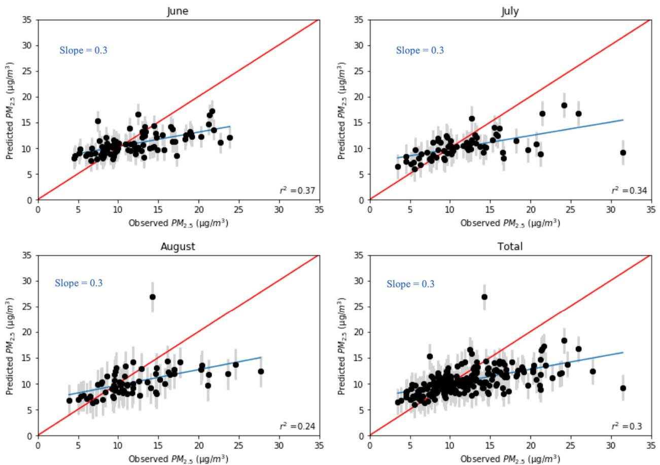
**Figure 8.** Scatter plots for Catawba County indicating model performance. The black points indicate the modeled versus predicted point, and the grey bars indicate the ±1 standard deviation of the modeled dataset. The red line indicated the one-to-one line and the blue line is the best fit line for the dataset. The slope of the best fit line is indicated in blue in the corner of each figure.
