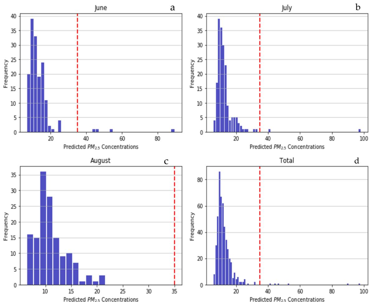
**Figure 9.** Histogram plot illustrating the model predictions in Sampson County for June (a), July (b), August (c) and total (d). The blue lines indicate the number of times (y-axis) the  $PM_{2.5}$  concentrations reached a certain amount (x-axis). The red line indicates the NAAQS exceedance value.
