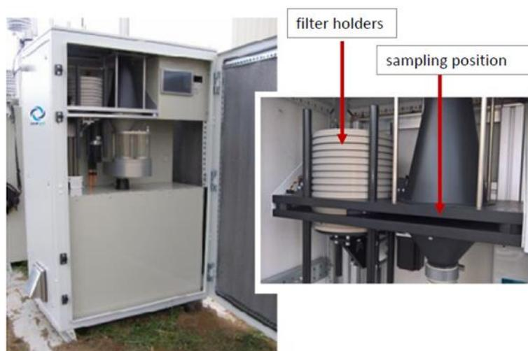
**Figure 2.** The high-volume sampler SAM Hi 30 AUTO WIND.
