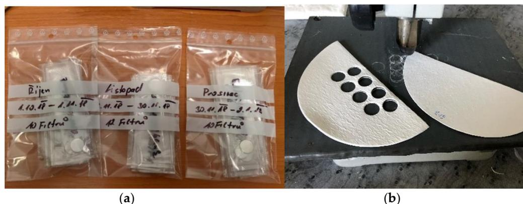
**Figure 4.** (a) A packed set of exposed filter samples, and (b) the preparation of samples using the special automatic punching head.
