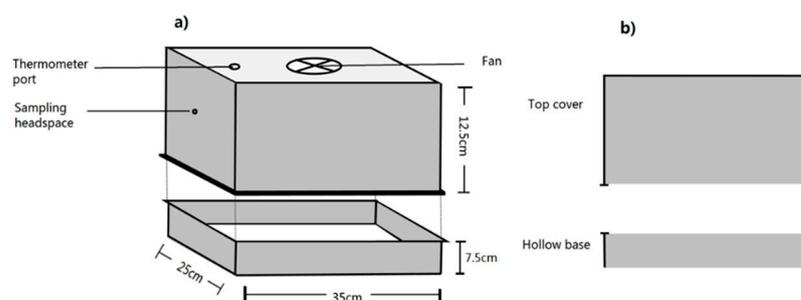
**Figure 2.** Schematic diagram showing the chamber design. Illustration (a) shows a three-dimensional hollow base and a top with a top while illustration (b) shows a transverse section of the base and the top cover.
