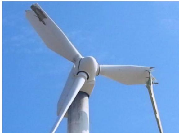
**Figure 3.** Photograph showing blade damage due to Typhoon Usagi [23].
