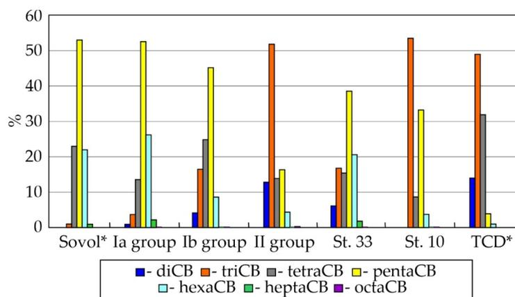
**Figure 5.** The PCB homological patterns (%) in groups obtained by the cluster method in comparison to homological patterns in technical mixtures of PCB (Sovol and trichlorodiphenyl (TCD); \* [61]).
