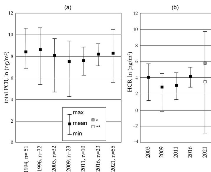
**Figure 2.** The comparison of the total PCB (a) and HCB (b) levels in snow from the 1990s to the 2020s (ln (ng/m<sup>2</sup>)) (\* mean HCB levels including data for Site # 31 near the industrial area of Usol'ekhimprom; \*\* mean HCB levels without data for Site # 31) [16,21–24], and present study.
