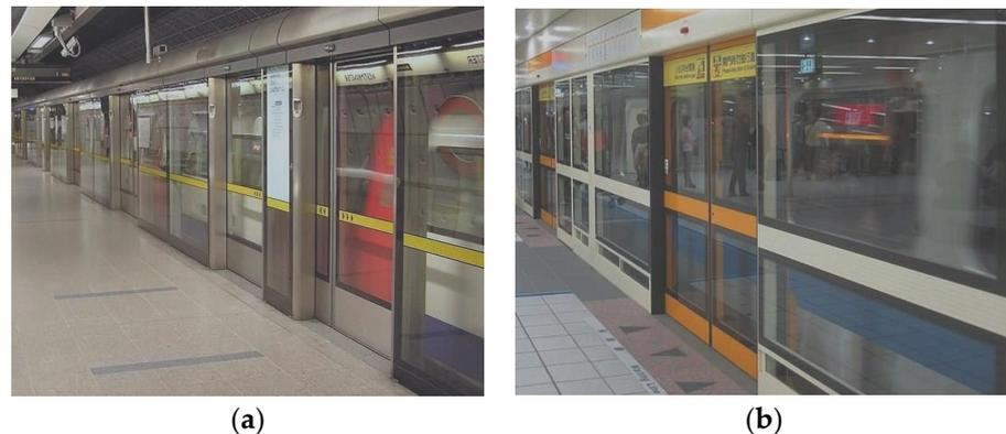
**Figure 1.** Practical PSDs with gaps on platforms. (a) single open door PSD; (b) double open door PSD.
