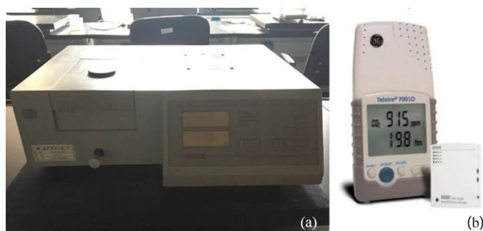
**Figure 1.** Test equipment: (a) spectrophotometer, (b) Telaire 7001 and HOBO.**Table 3.** Equipment information.
