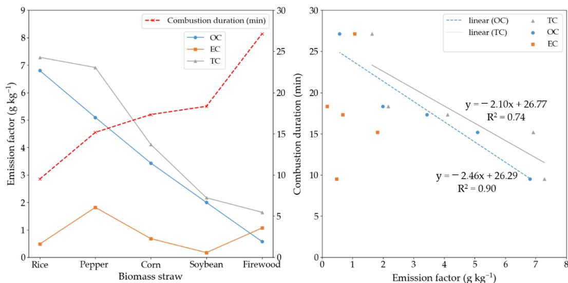
**Figure 3.** (a) Emission factors for OC, EC, and TC from the five types of biomasses, and (b) combustion durations for the five types of biomasses.
