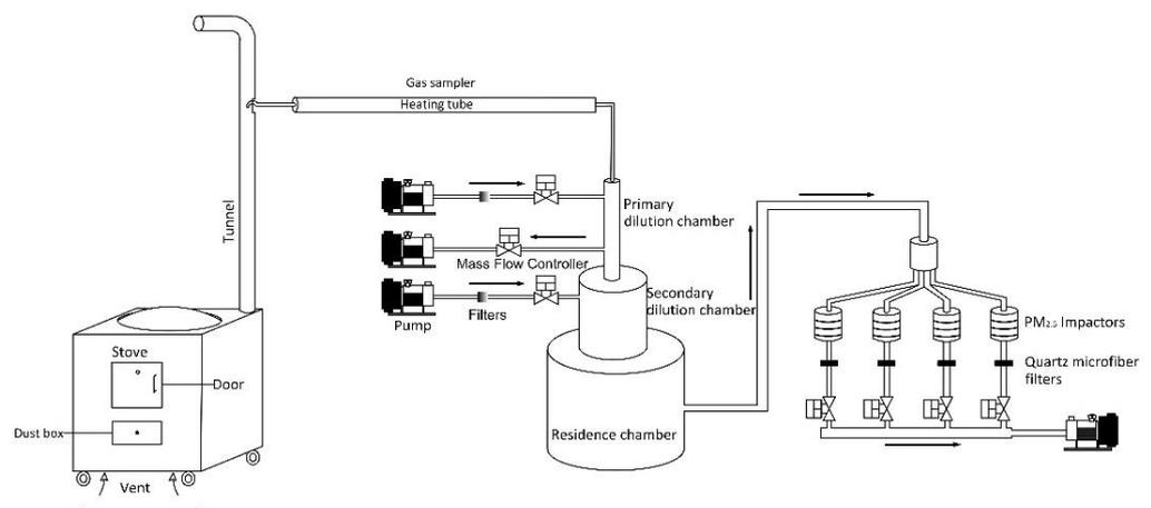
**Figure 2.** Sketch of the diluting and sampling system.
