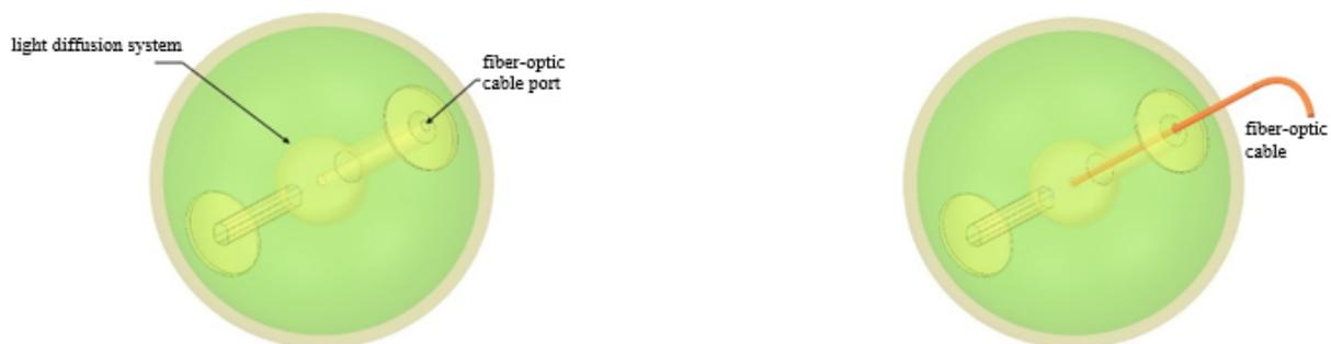
**Figure 14.** Proposed method for inserting and fitting fiber-optic cables into capsules.
