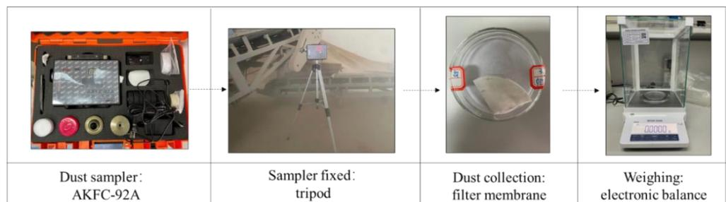
Figure 2. Dust concentration measuring instrument.
