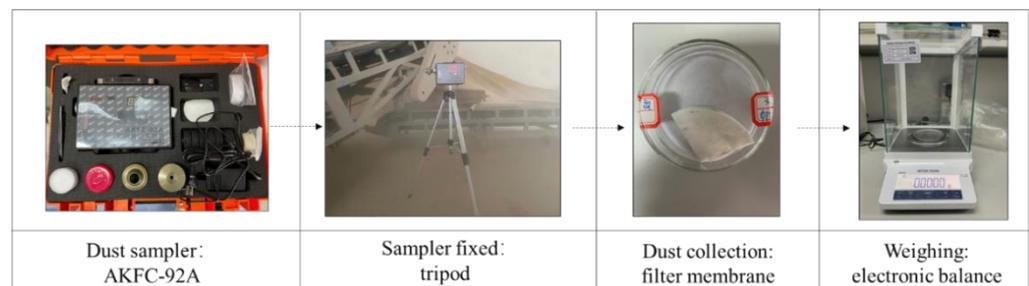
Figure 2. Dust concentration measuring instrument.
