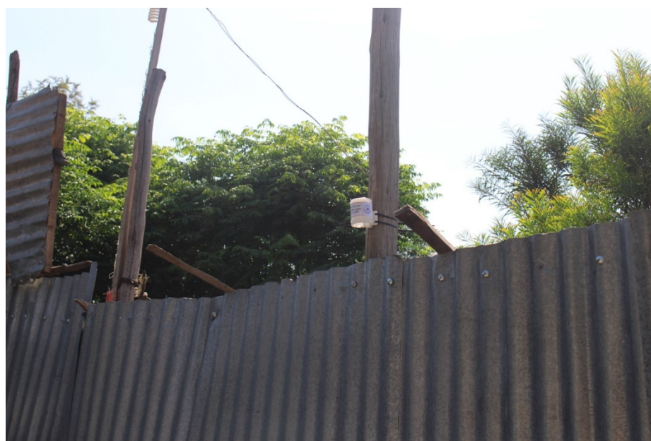
Figure 2. Photo of Ogawa badge in its rain protection from one of the \text{NO}_x and \text{NO}_2 sampling sites.
